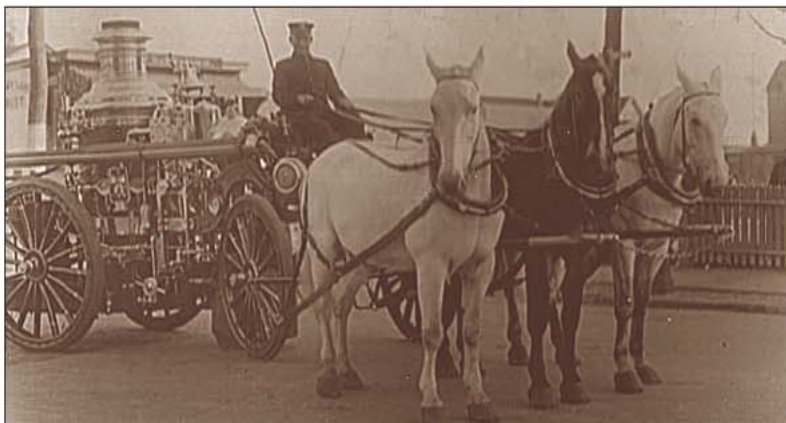
Fig. 1-1. Horse-drawn steam fire engines were used from the 1860s to the 1920s.
