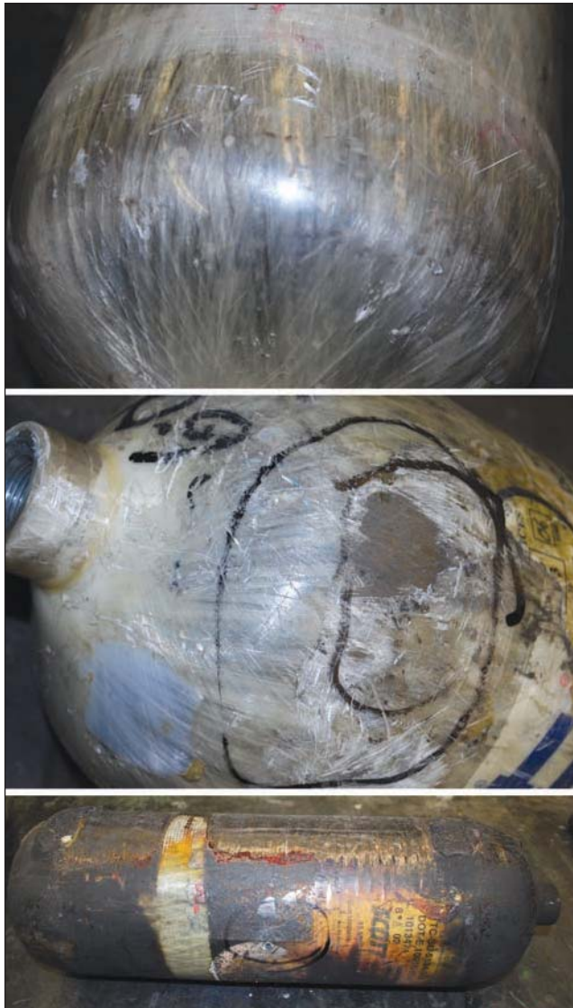
Fig. 10-15. Examples of Level 1, Level 2, and Level 3 damage
