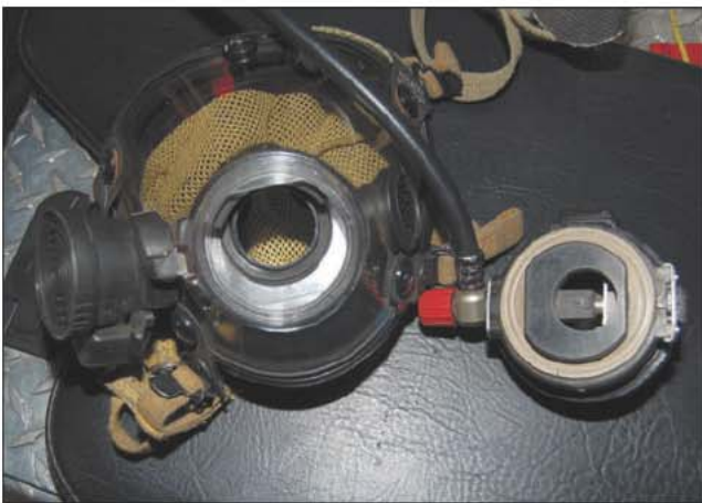
Fig. 10–20. The mainline valve on this MMR is internal and operates automatically. The bypass valve is red and can be seen mounted on the left side of the MMR.
