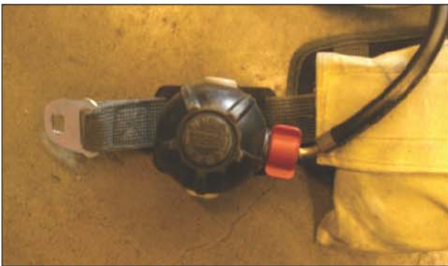
Fig. 10–19. The MMR shown here is properly stored. When placed in service, the regulator is attached to the facepiece.
