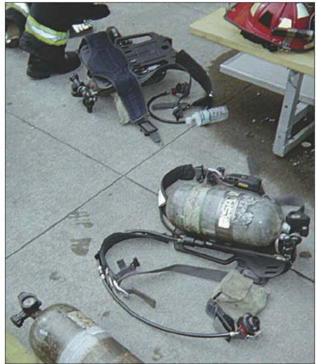
Fig. 10–27. Two SCBA temporarily stored on the ground with the regulator exposed. Improper storage can result in water or debris entering the regulator assembly and causing a malfunction. Always store the SCBA with the regulator protected.
