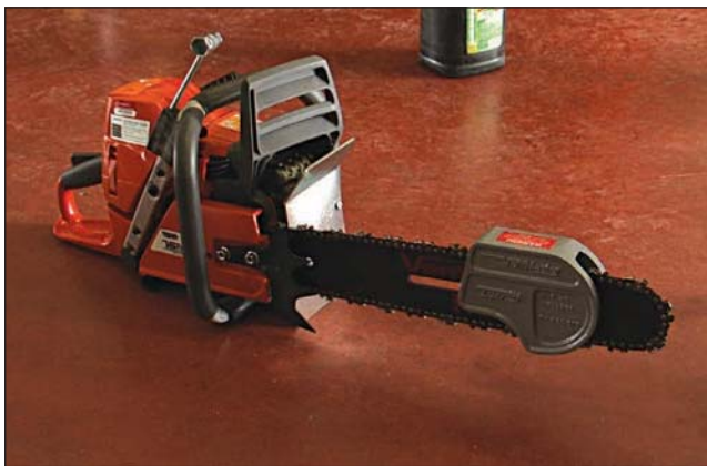
Fig. 11–31. A chain saw with a depth gauge
