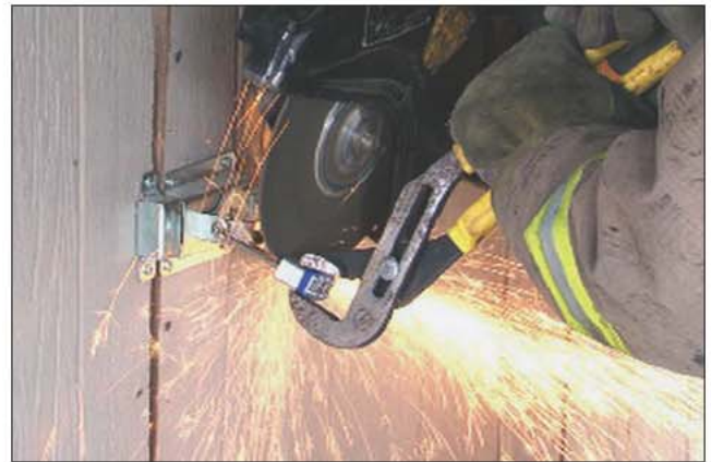
Fig. 11–26. One firefighter cuts a padlock while another firefighter holds the padlock with a pair of channel locks.
