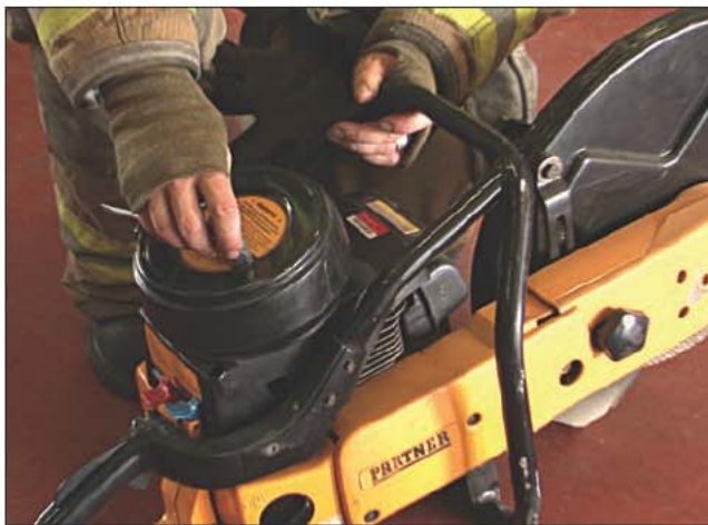
Fig. 11–28. Make sure all nuts and bolts are secure.
