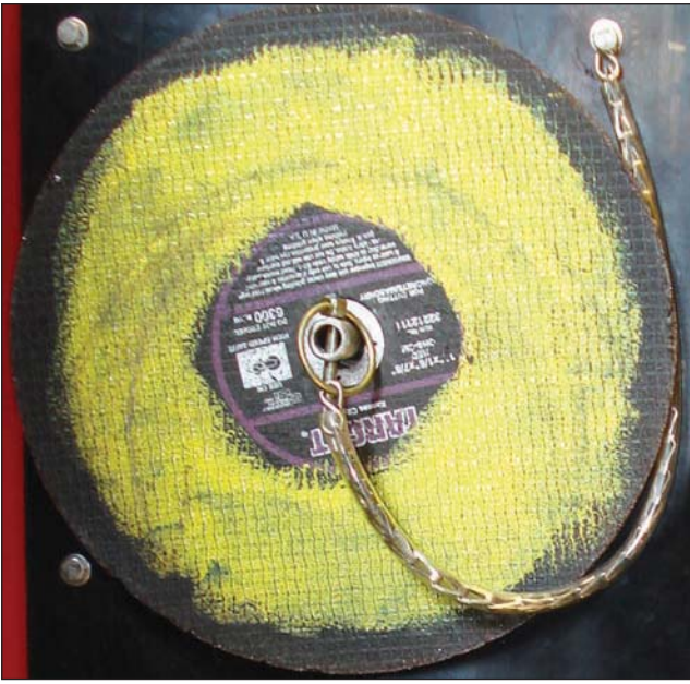
Fig. 11–21. The aluminum oxide and silicone carbide abrasive blades are similar in appearance, some departments paint the blade yellow to distinguish the two.
