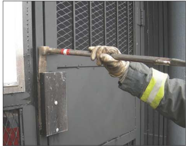
Fig. 12–28. The use of a Halligan tool on an ornamental entry gate
