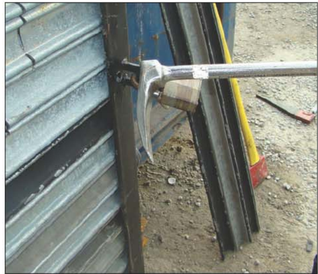
Fig. 12–14. Halligan tool breaking padlock
