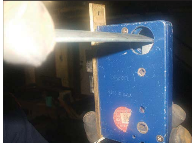
Fig. 12–18. Demonstrating the use of a key tool on a mortise lock
