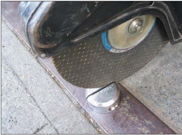
Fig. 12–16. Firefighter cutting American Lock Series 2000 lock with power saw
