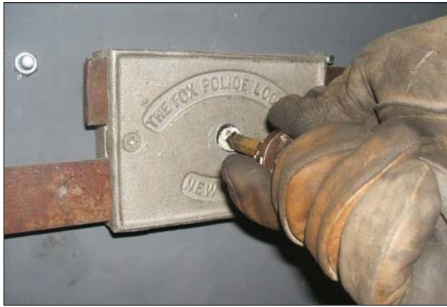
Fig. 12–25. Opening a fox lock with 5/32 square tool
