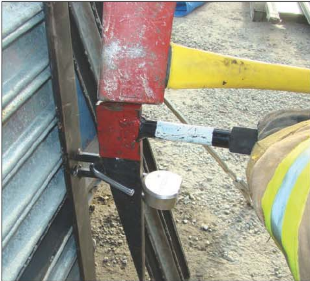
Fig. 12–13. Duck bill breaking heavy-duty padlock
