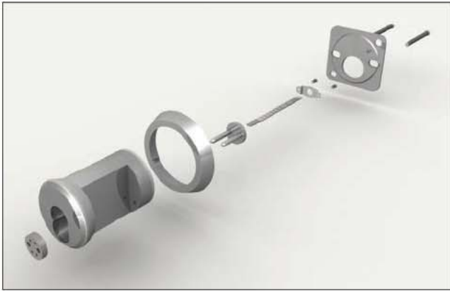
Fig. 12–21. An exploded view of a key-operated rim lock
