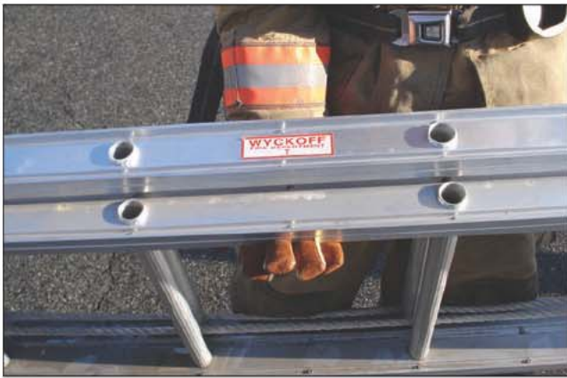
Fig. 13–12. A sticker marking the balance point
