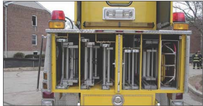
Fig. 13–30. Vertical ladder storage. (Courtesy of S. K. Willis)
