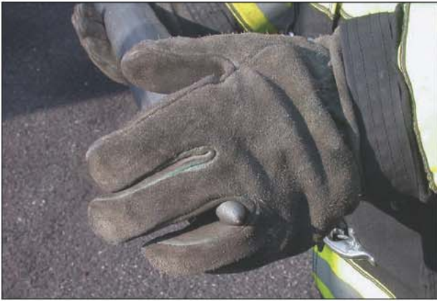
Fig. 13–96. Keep the spur between your fingers as you raise the ladder.
