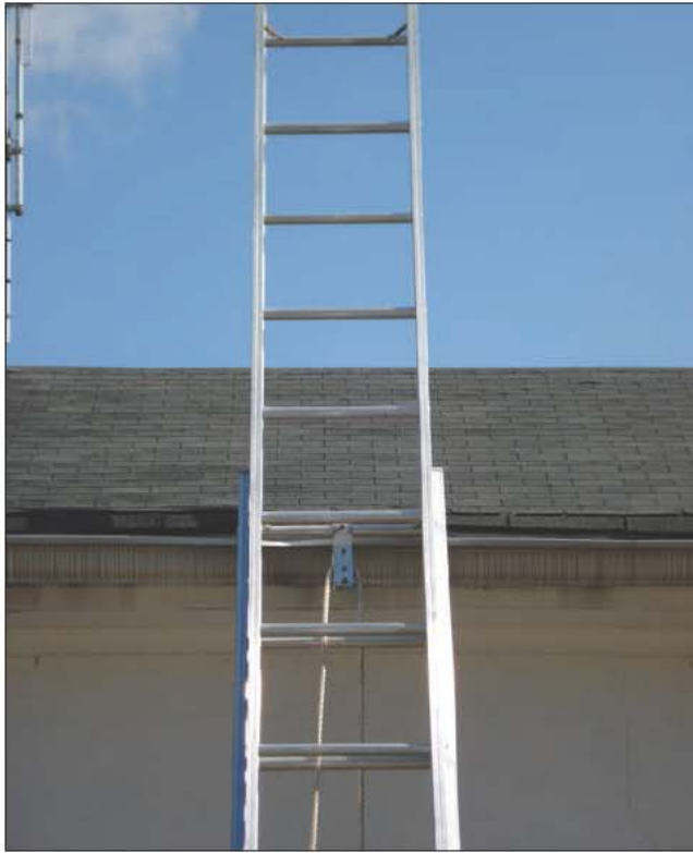
Fig. 13–65. The ladder should extend five rungs above roof level.
