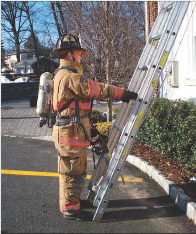
Fig. 13–41. Quick method to check ladder angle
