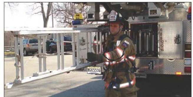
Fig. 13–35. Find the balance point and carefully remove the ladder.
