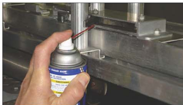
Fig. 13–21. Lubricating the dogs
