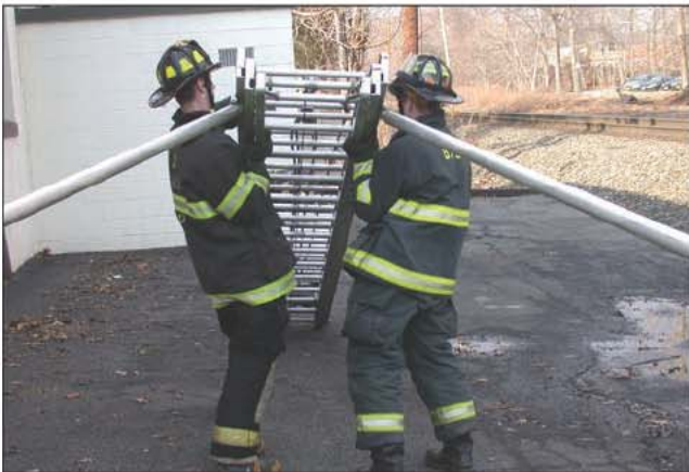
Fig. 13–97. Two firefighters at the tip, one at the base, and two on the poles.
