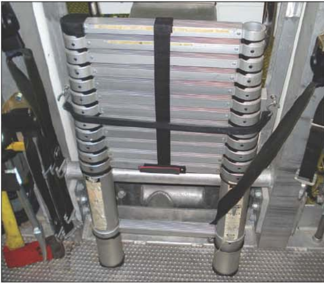
Fig. 13–38. Collapsible ladder mounted inside tower bucket
