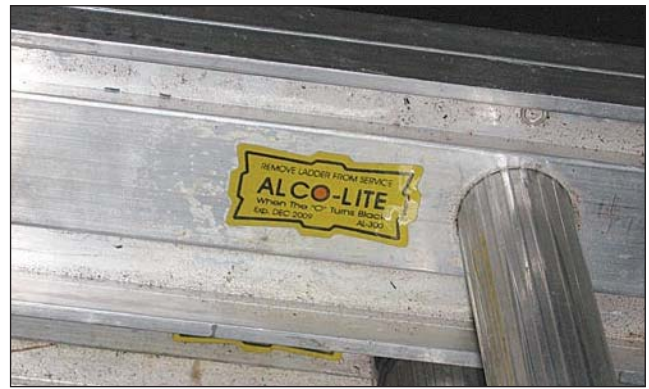
Fig. 13–17. A heat sensor sticker notifies firefighters when the ladder has been exposed to high heat.
