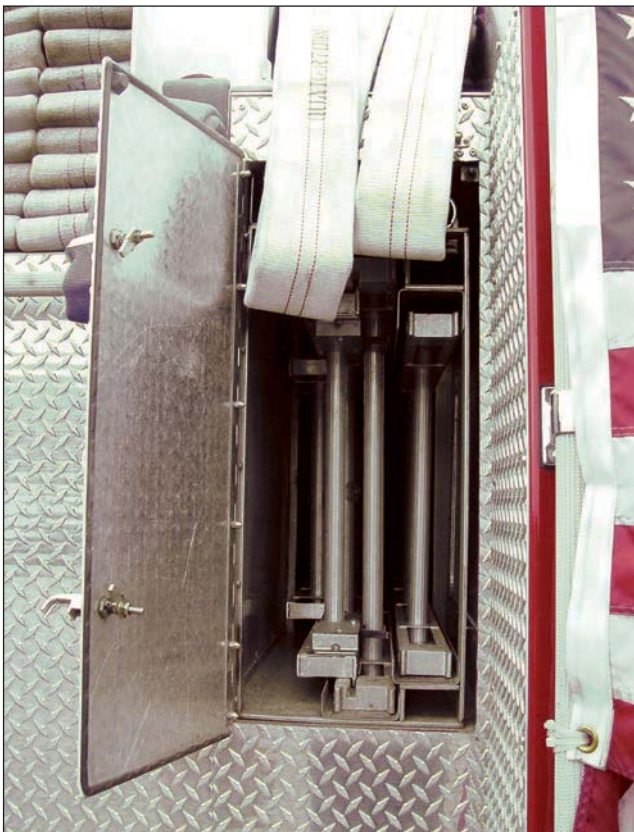
Fig. 13–24. A vertical ladder-storage compartment. (Courtesy of S. K. Willis)
