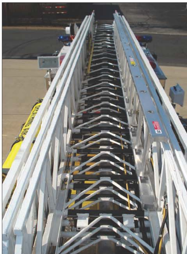
Figs. 13–36. Roof ladder mounted on aerial
