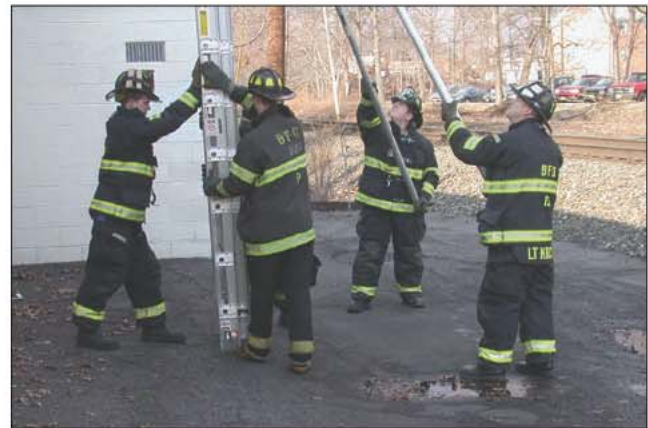
Fig. 13–98. One support pole to the side and another toward the center stabilize the ladder.
