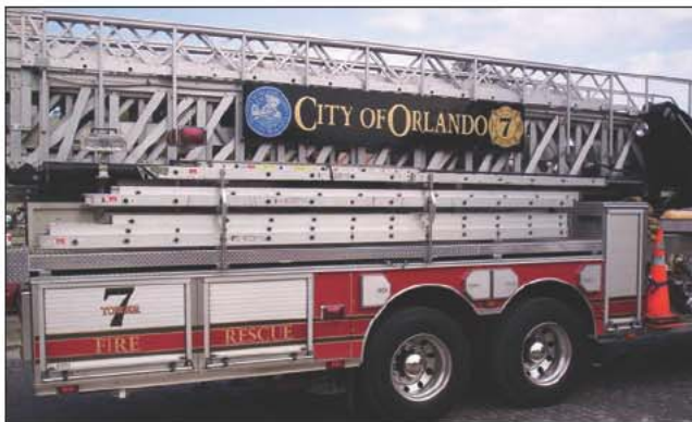
Fig. 13–32. Ladders stored on side compartment racks
