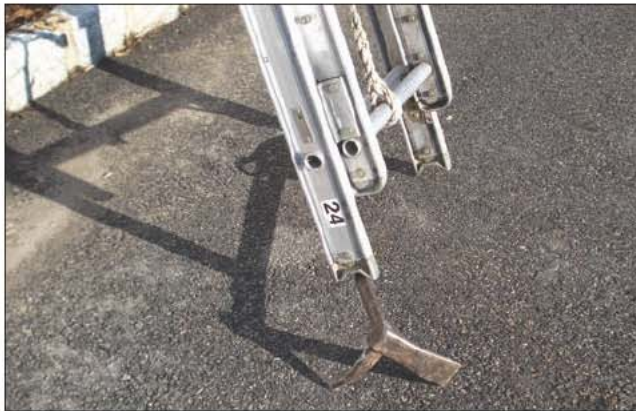
Fig. 13–40. Halligan used as ladder support
