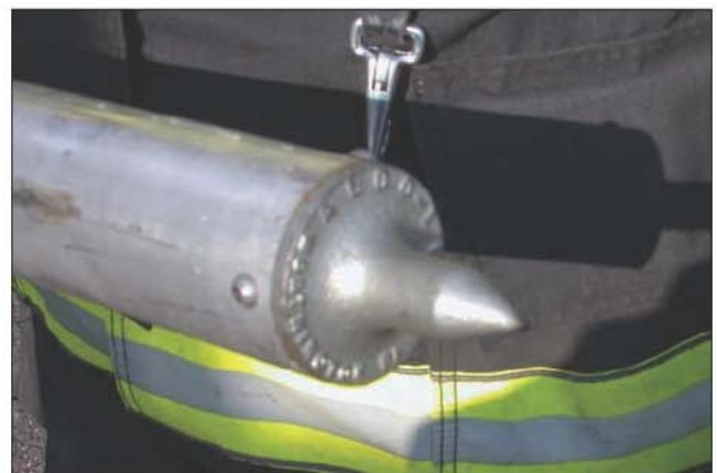
Fig. 13-95. There is a sharp spur at the base of the poles.
