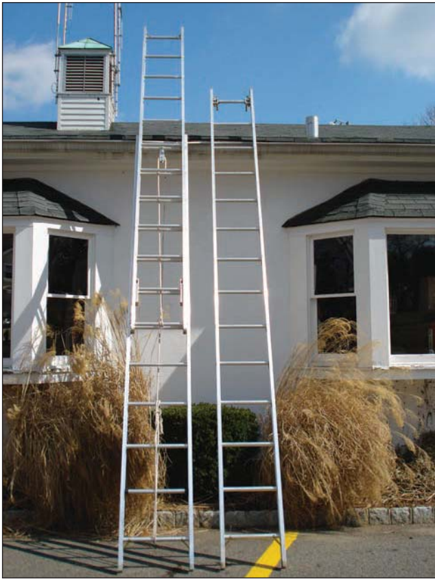
Fig. 13–7. An extension ladder and a roof ladder
