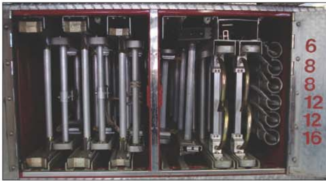
Fig. 13–31. Ladder with hooks toward the rear of the compartment
