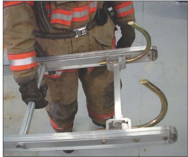
Fig. 13–6. Roof ladder with hooks deployed
