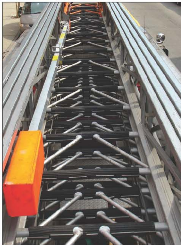
Fig. 13–37. Folding ladder mounted inside aerial
