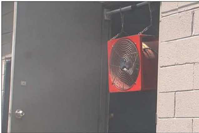
Fig. 14–12b. A smoke ejector placed in a doorway to remove smoke via negative pressure ventilation
