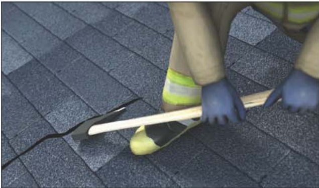
Fig. 14-42. An axe head that is trapped below roof decking can be levered out by placing the toe of your boot between the roof and the junction of the head and handle.
