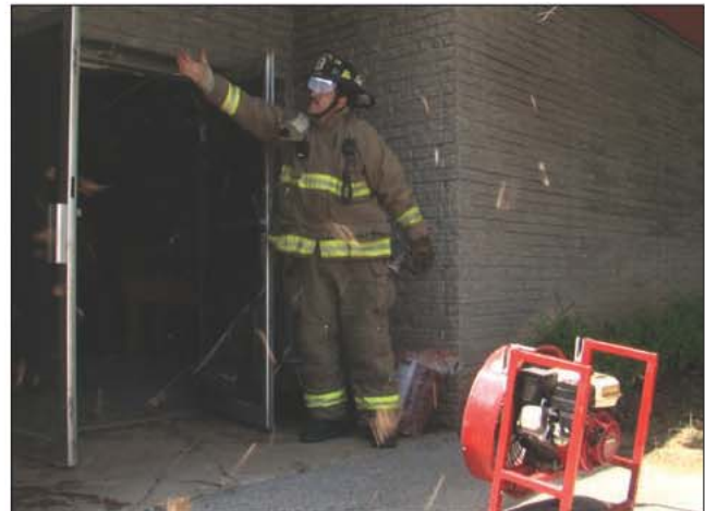
Fig. 14–8. A firefighter has set up a PPV fan and checks to ensure that the entire doorway is covered by the flow of air into the building.
