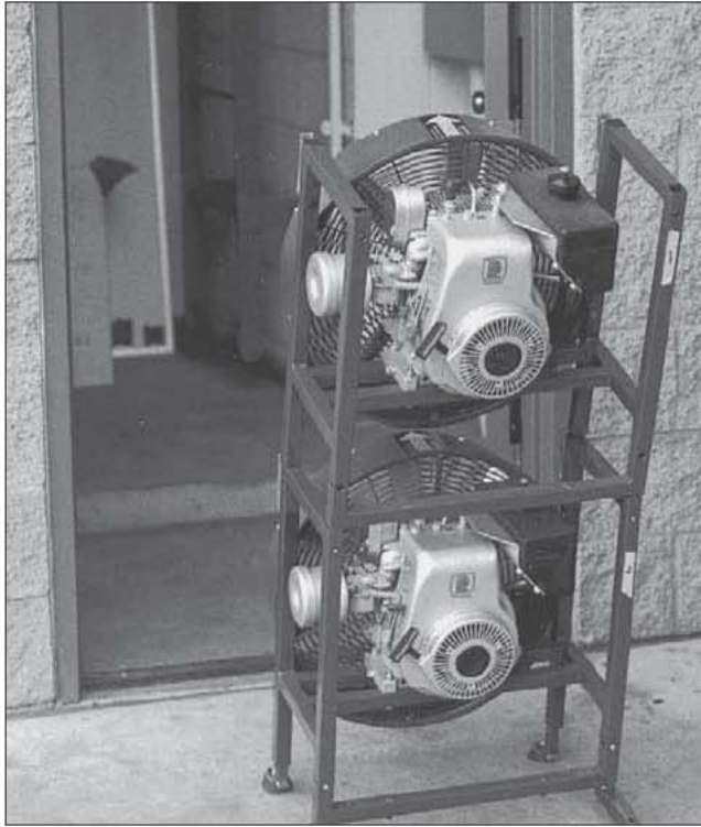
Fig. 14–12a. Various tools may be used to perform both positive and negative ventilation, such as fans, blowers, smoke ejectors, and fog streams.
