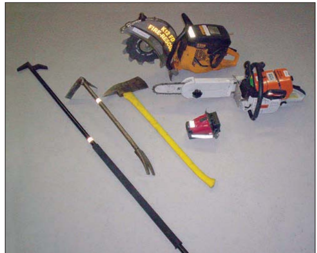
Fig. 14–41. These are various tools that can be very useful for roof ventilation operations. It is important to understand the strengths and weaknesses of various ventilation techniques.
