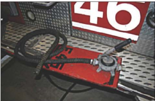
Fig. 15–16. Dry barrel hydrant pump
