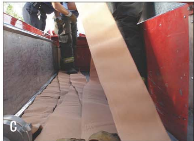
Fig. 15–74 a, b, c. Firefighters load 800 ft (244 m) of 4-in. (100-mm) hose in a flat load. This 4-in. (100-mm) NST LDH is set up for a forward lay with the female coupling out.
