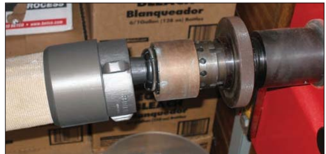
Fig. 15–27b. Hose mounted with coupling expander
