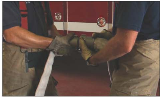
Fig. 15–29. Firefighters utilize various techniques to aid in coupling and uncoupling hose.
