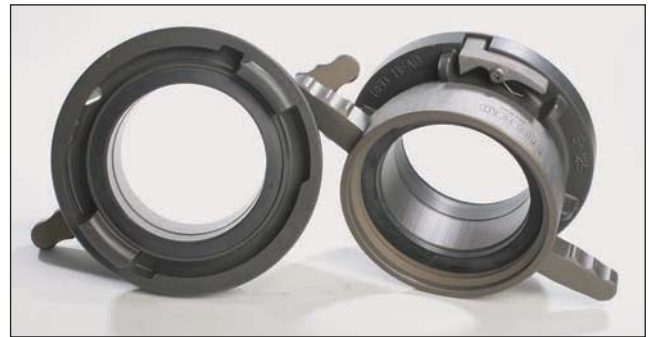
Fig. 15–38. Storz adapter: 5-in. (125-mm) Storz locking to 4½-in. (115-mm) female swivel, extended lug. (Courtesy of Adam Weidenbach)
