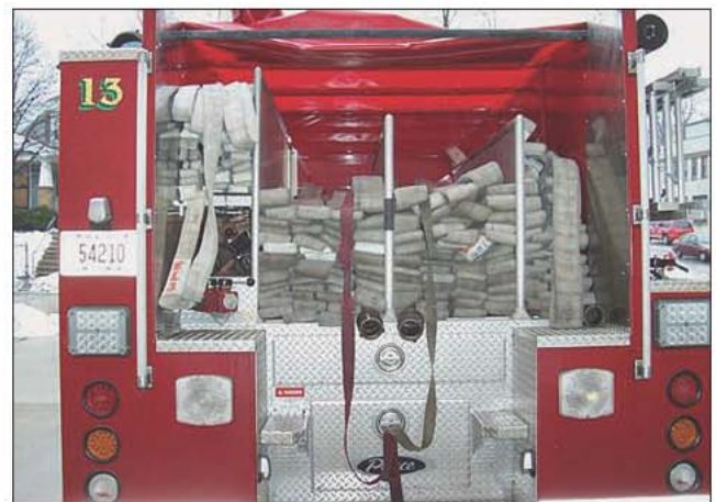
Fig. 15–79 MFD hosebed setup for reverse lays
