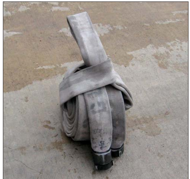
Fig. 15-73. Self-locking twin donut roll
