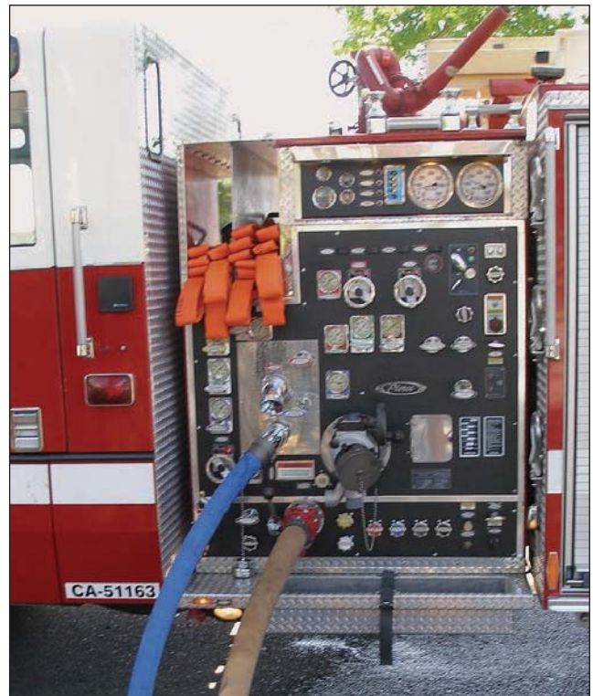
Fig. 15–63. Preconnected attack crosslays. (Courtesy of Daryl Liggins)
