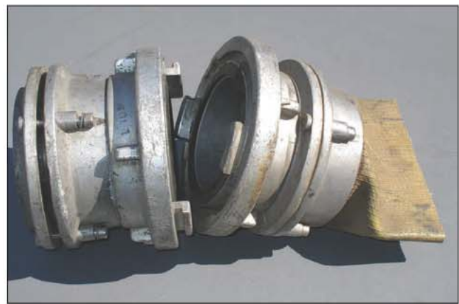
Fig. 15–30. Nonlocking 5-in. (125-mm) Storz coupling
