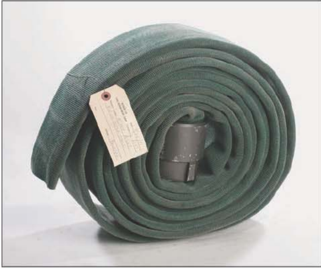
Fig. 15–60. Out-of-service hose, male coupling removed, with properly filled-out and attached repair tag. (Courtesy of Adam Weidenbach)
