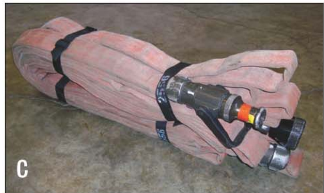
Fig. 15–69 a, b, c. Horseshoe hose bundles of 50 ft (15 m) and 100 ft (30 m). (Courtesy of Daryl Liggins)
