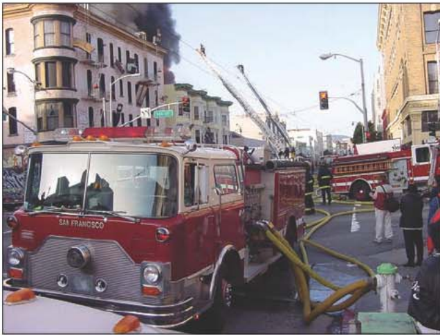
Fig. 15–80. SFFD pumps dual 3-in. (75-mm) MDH lay at hydrant
