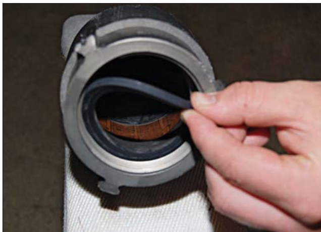
Fig. 15–32. It is important to check hose gaskets for wear and tear, on a regular basis.
