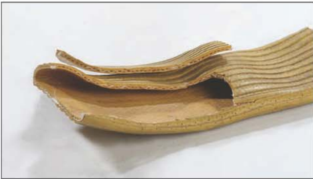
Fig. 15–25. Extruded 1½-in. structure fire hose. (Courtesy of Adam Weidenbach)
