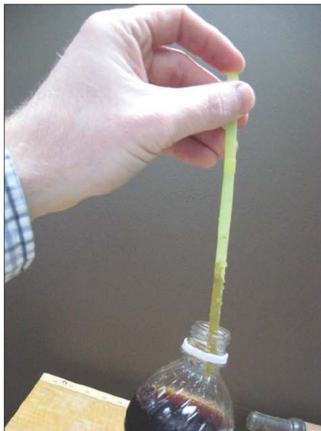
Fig. 15–3. A simple way to demonstrate atmospheric pressure is with liquid and a straw.
