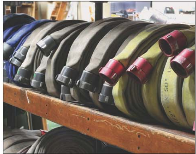
Fig. 15–62. In-service hose properly stored on a hose rack. (Courtesy of Adam Weidenbach)
