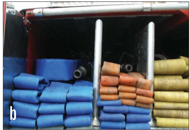
Fig. 15–67 a, b. Static attack lines loaded in the hosebed. (Photos courtesy of Daryl Liggins)
