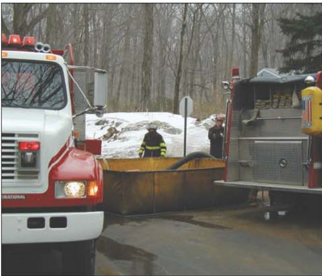
Fig. 15–18. A simple water shuttle operation can effectively supply water for fireground operations.
