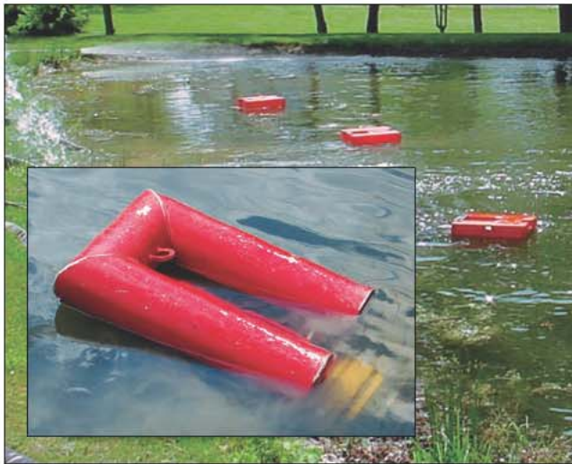
Fig. 15–82. Floating strainer in operation
