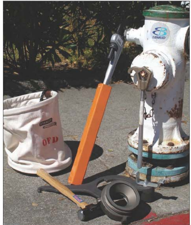
Fig. 15–85. An example of tools in a hydrant bag
