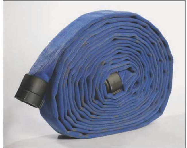
Fig. 15–58. In-service straight roll, with male-threaded coupling protected. (Courtesy of Adam Weidenbach)
