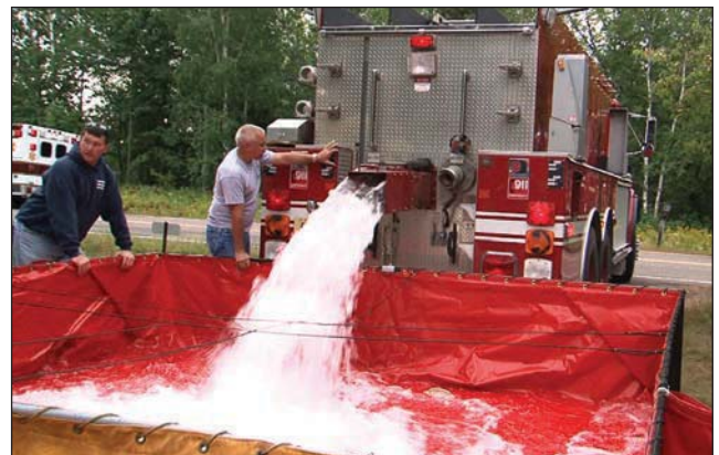
Fig. 15–17. Most water tenders have an easily deployable, folding, portable water tank.
