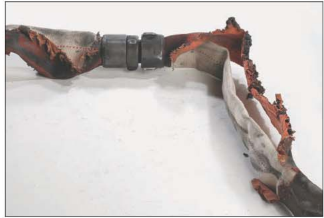
Fig. 15–61. Severely damaged 1 \frac{3}{4} -in. (45-mm) DJ hose. Cut the couplings off and discard hose. Do not roll. (Courtesy of Adam Weidenbach)
