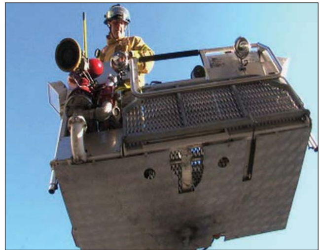
Fig. 16–41. A tower ladder water monitor and control valve
