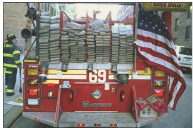
Fig. 16–13. A bed of supply hose on the left and three beds of static attack hose loads. Static loads are not preconnected and are also known as dead loads. (Photo by Jay Comella)
