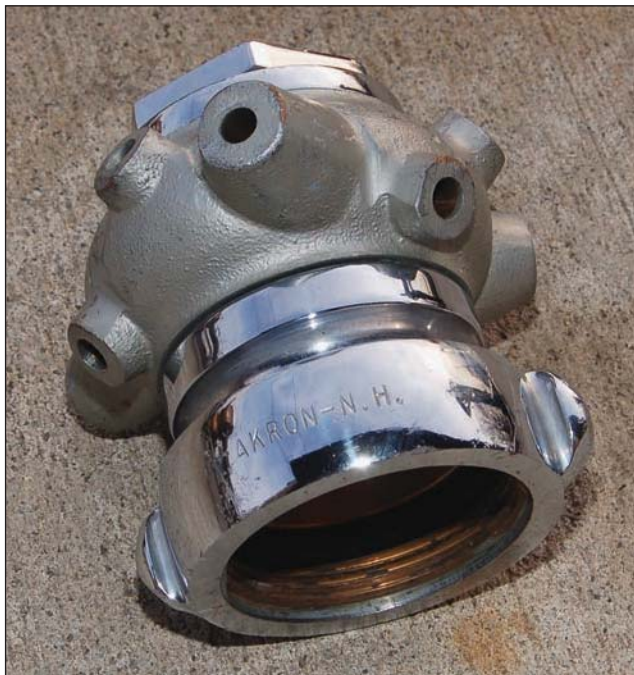
Fig. 16–45. A Bresnan distributor is used primarily for basement fires where normal fire attack is not possible.
