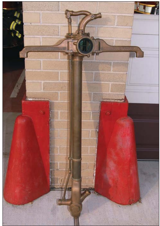
Fig. 16–46. Cellar pipes have a directed stream that can be pointed in any direction underneath a floor.
