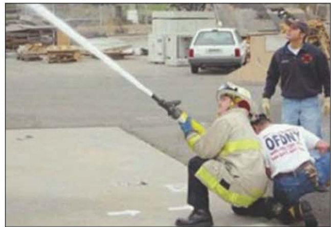
Fig. 16–5. California's Oakland Fire Department (OFD) members operate a 2\frac{1}{2} -in. (65-mm) hoseline with a \frac{1}{8} -in. (30-mm) smooth bore nozzle (266 gpm at 50 psi [1,007 L/min at 345 kPa]) during testing and evaluation. (Courtesy of Daryl Liggins)
