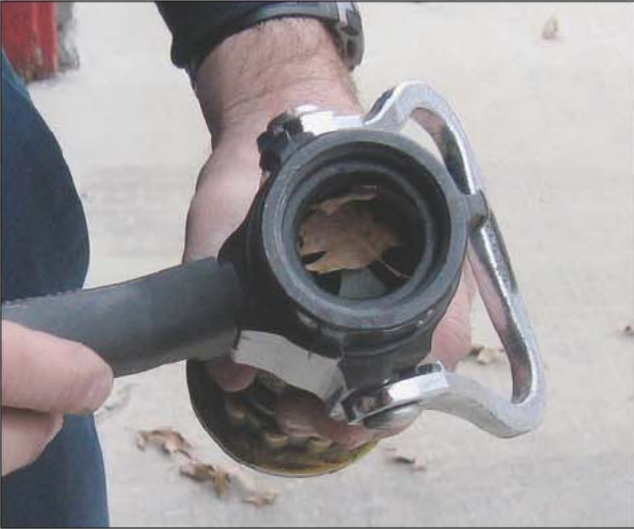
Fig. 16–47b. A blocked waterway inside a nozzle
