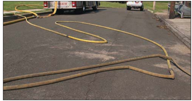
Fig. 16–15. Kinked lines prevent maximum flow of water to the fire.
