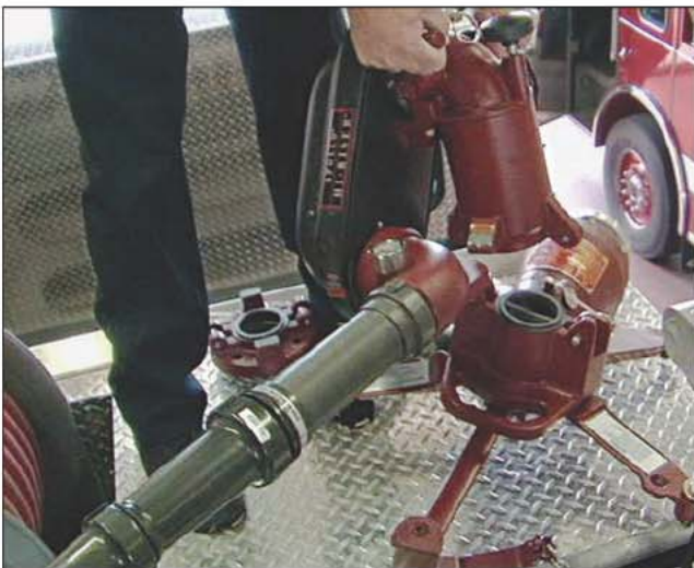
Fig. 16–42d. Attaching nozzle to base
