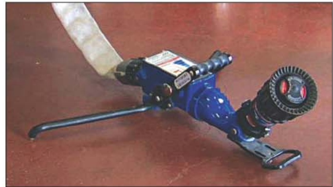
Fig. 16–43. A non-apparatus mounted deluge gun is a portable monitor that is always used on the ground.
