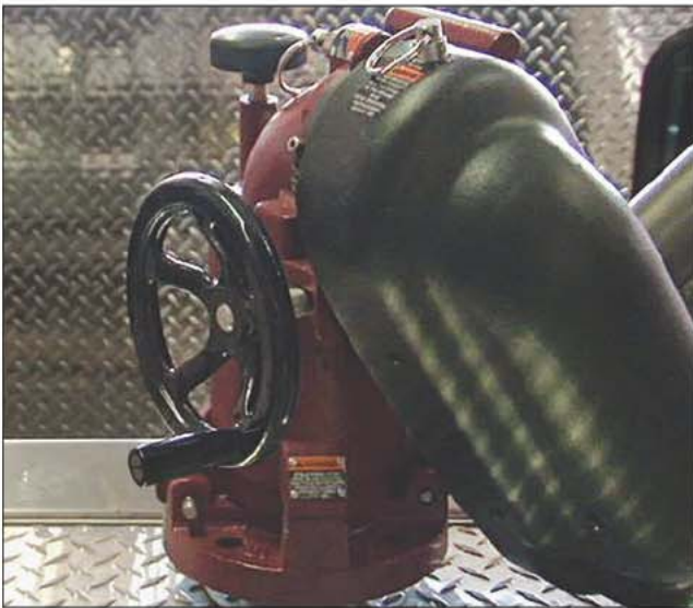
Fig. 16–42c. Handle to raise and lower nozzle
