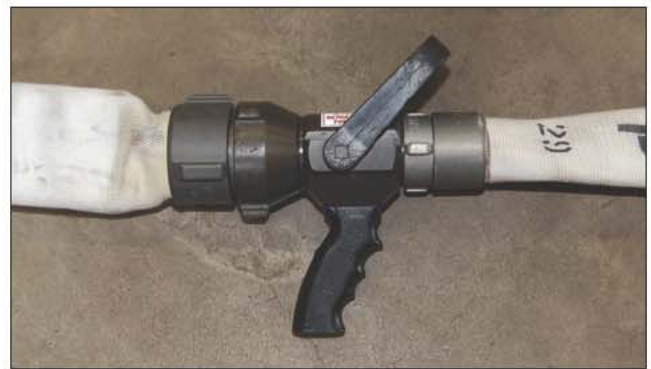
Fig. 16–37. The stack tips on a 2 1/2-in. smooth bore nozzle can be removed allowing a smaller hoseline to be attached. The 2 1/2-in. then functions as a gate valve.
