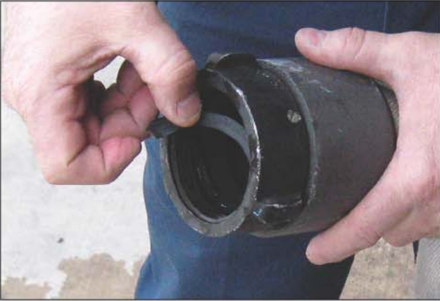
Fig. 16–47c. Replacing a worn out gasket in a nozzle
