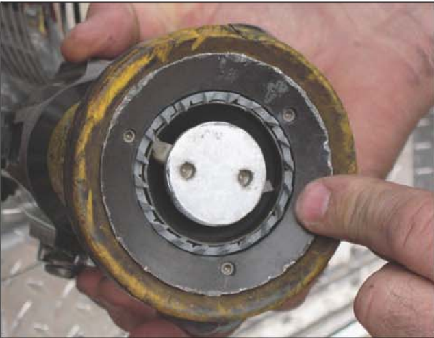
Fig. 16–47a. Nicks and dents on a nozzle
