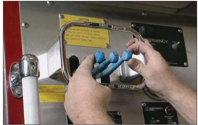
Fig. 16–40c. Electronic controls for ladder pipe
