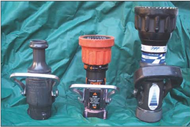
Fig. 16–3. Left to right: \frac{1}{16} -in. (24-mm) smooth bore nozzle (180 gpm at 50 psi [681 L/min at 45 kPa]), constant gallonage nozzle (150 gpm at 50 psi [568 L/min at 345 kPa]), and an automatic nozzle (50–300 gpm [189–1,136 L/min]). (Courtesy of Jerry Knapp)
