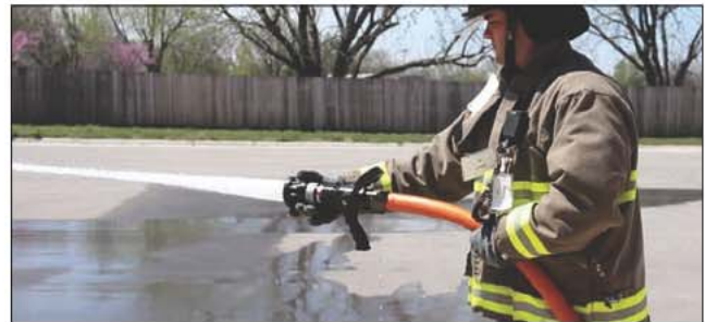
Fig. 16–7e. Fog nozzle adjusted to straight stream
