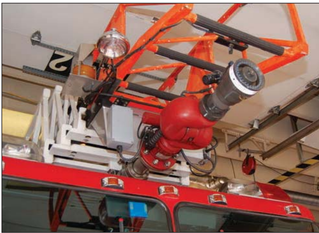
Fig. 16–40a. A permanently mounted ladder pipe
