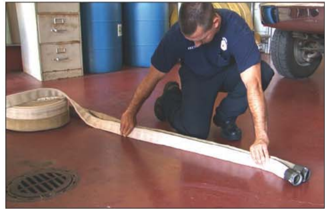
Fig. 16–1. The 1¾-in. (45-mm) hose allows significantly higher flow than the 1½-in. (38-mm) line, yet size and weight differences are nominal.
