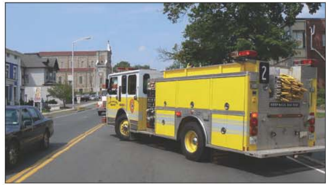
Fig . 17–29. Apparatus blocking an accident scene with its wheels turned away from personnel working on scene. (Courtesy of firegroundimages.com)
