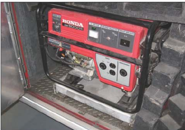
Fig. 17–30. A gas powered portable generator. (Courtesy of Lou Tibor)
