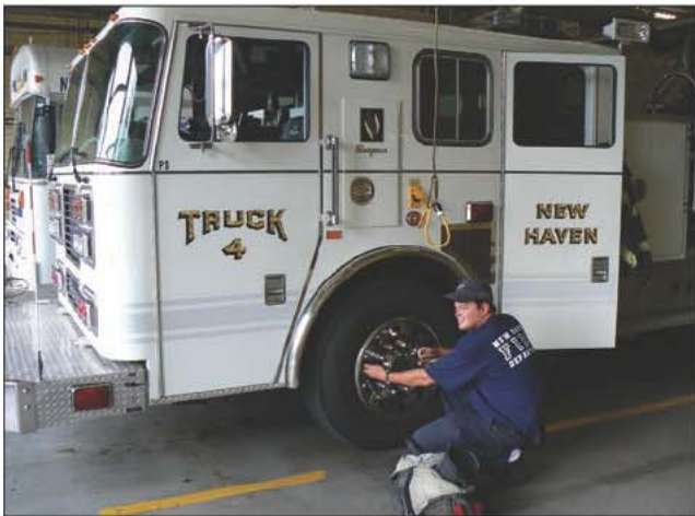
Fig. 17–27. A firefighter conducts a pre-trip inspection at the start of his shift to ensure the safety of his crew.
