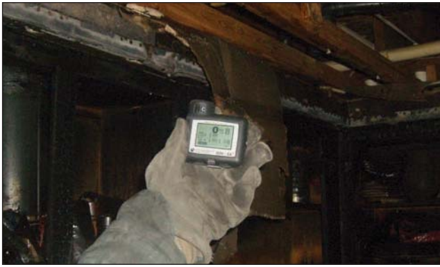
Fig. 17–72. Firefighters should meter the atmosphere before removing SCBA. Remember that the consequences of exposure may, in the long term, result in stroke, heart attack, and cancer.
