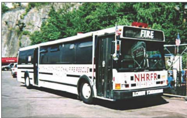
Fig. 17–8. This rehabilitation and care (RAC) unit is a converted passenger bus. It was modified and reequipped to serve as a rehab unit.
