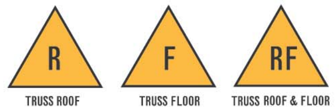
Fig. 17–68. Triangle markings indicating the presence of trusses
