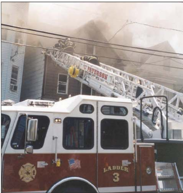
Fig. 17-4. All equipment should be kept at least 10 feet from power lines. Operations here show a reprehensible disregard for safety. (Courtesy of Ron Jeffers)
