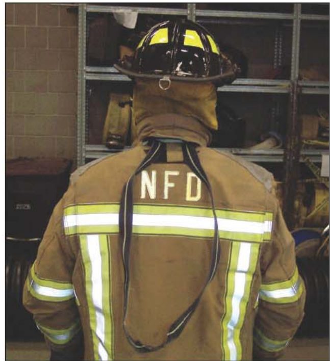
Fig. 17-91. The drag rescue device (DRD) deployed. (Photo by Jim Ricci, courtesy of Globe)
