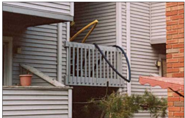
Fig. 17–59. Hoseline management must be a top priority. Water equals protection for everyone. No one should ever pass a kink. (Courtesy of Ron Jeffers)
