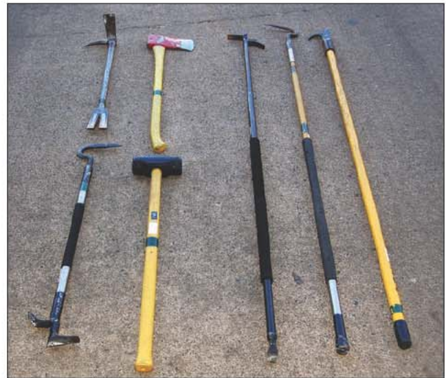
Fig. 19–1. Search tools come in a wide variety of shapes and sizes. Many commonly used tools were actually developed by firefighters looking for innovative ways to combine or improve standard tools.
