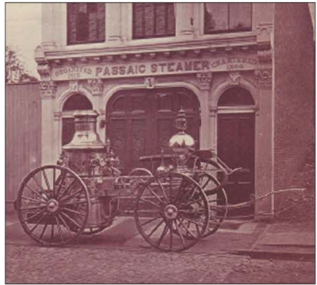
Fig. 2–6. A beautiful steam fire engine of the Passaic Engine Company Number One of Paterson, New Jersey. This heavy, hand-drawn “steamer” was built in 1874.
