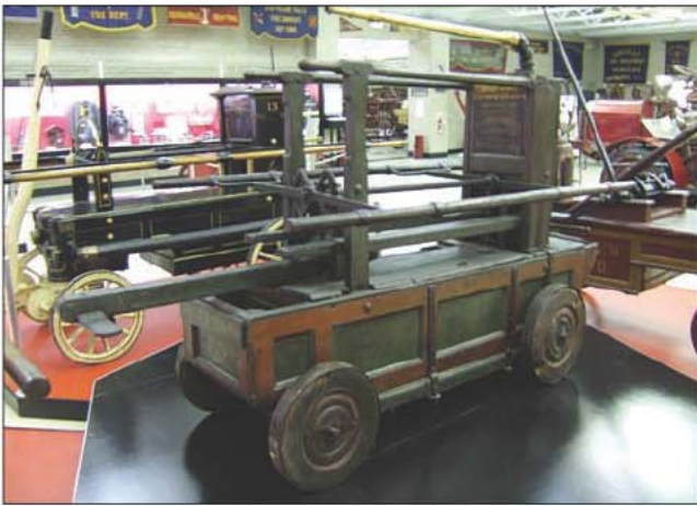
Fig. 2–2. One of two Newsham engines New York City imported in 1731 from London, now on display in the American Museum of Firefighting in Hudson, New York. The two wooden handles on the sides of the engine—called “brakes”—were lifted up and down to pump the engine.
