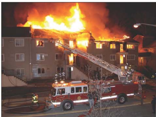
Fig. 20–18. This is a good example of a fire that needs large lines. There is a greatly advanced body of fire, necessitating a defensive operation, and at this point it is still undermined how much of this building the fire will involve. The high heat production will require tons of water to extinguish the fire. (Courtesy of Brian Duddy)
