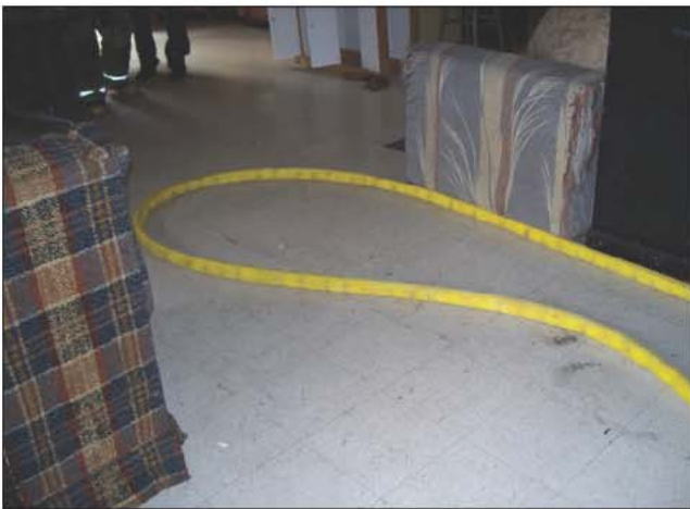
Fig. 20–42. Making a loop of hose on the floor allows the nozzle team to advance quickly and easily.
