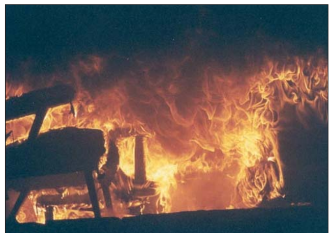
Fig. 20–47. This room has gone to flashover. The chair on the left and sofa on the right are fully involved almost to the floor level, and flames fill the entire room from floor to ceiling. Ceiling temperatures reach 2,000°F (1,093°C) or more.
