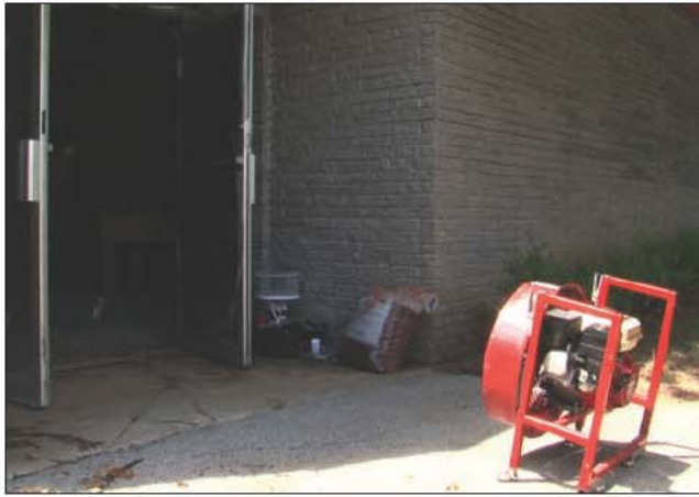
Fig. 20–56. A PPV fan placed at the front door will drive smoke and heat out horizontal ventilation openings created by firefighters. By controlling what windows are opened and closed firefighters can control the air flow through the building ventilating specific rooms as needed.
