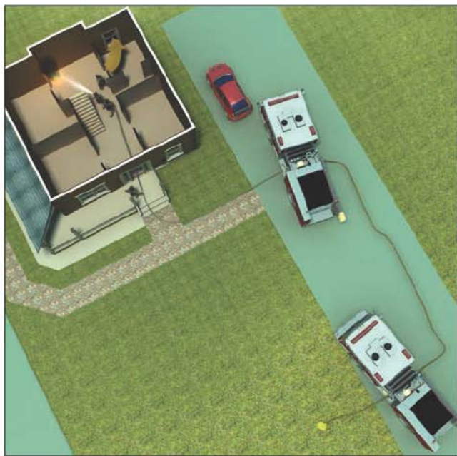
Fig. 20–11. Establishing a reliable water supply
