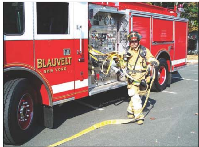
Fig. 20–31. The door position makes sure the hose bed is clear of all hose during the first part of the stretch.
