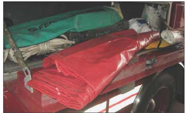
Fig. 21–4. While canvas salvage covers are found in most fire departments, they are being replaced by vinyl covers such as these.
