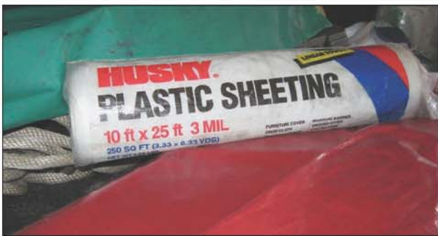
Fig. 21–6. Polyethylene plastic sheathing is a popular alternative to traditional salvage covers because of its low cost and the ability to manipulate its size.
