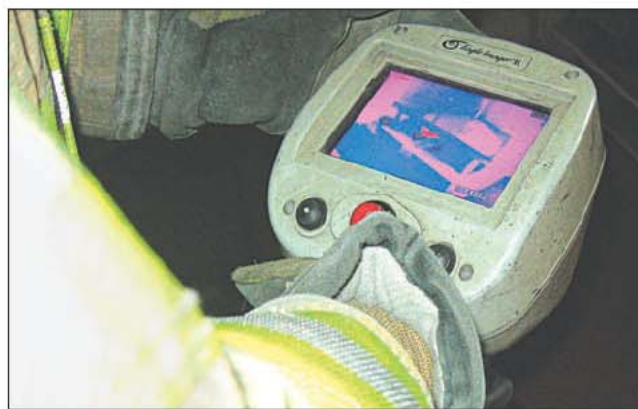
Fig. 21–18. Thermal imaging technology has allowed the overhaul process to be less damaging to property and more time efficient.
