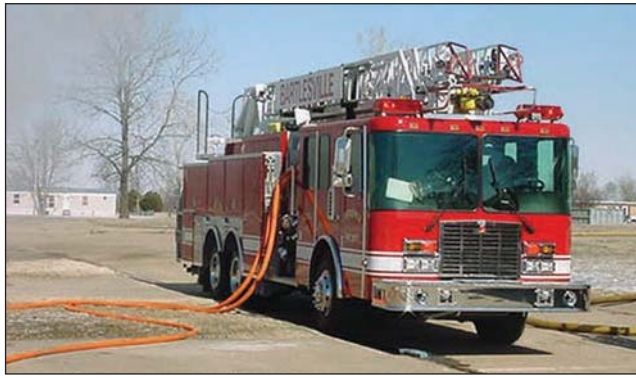
Fig. 3–9. Quints are combination units that can do the work of both engine and ladder companies since they have a fire pump, a water tank, hose storage area, aerial ladder, and ground ladders.
