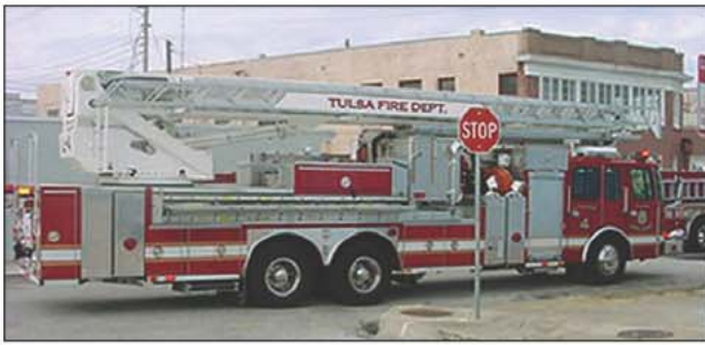
Fig. 3–6. A ladder or truck company. These units can come with a wide variety of fixed aerial devices.
