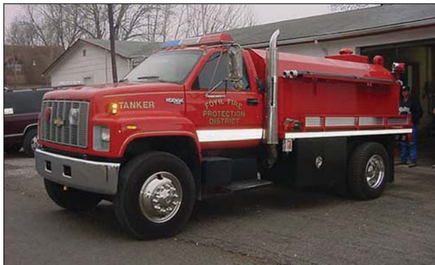
Fig. 3–10. Mobile water supply apparatus, commonly referred to as tenders, help fire departments fight fires in areas without fire hydrants.
