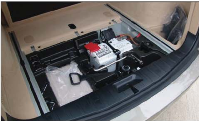
Fig. 34–41. Batteries may be found in many locations such as under the rear seat, behind the front driver-side fender, under the floorboard, or, as in the BMW X3, in the trunk.
