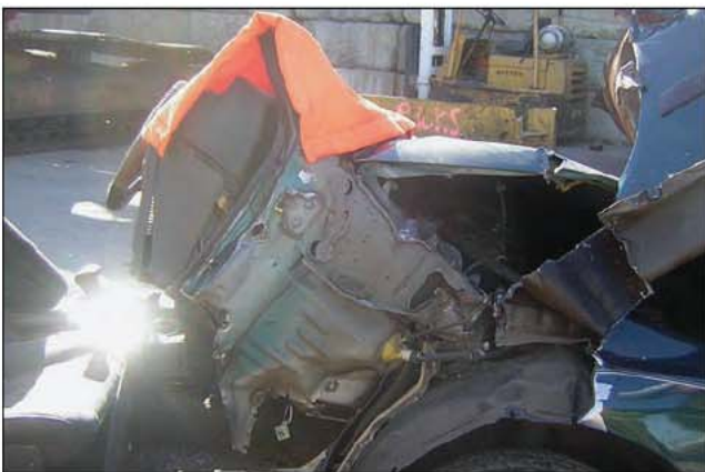
Fig. 34–68. This photo displays a side view of the dash lift end result.
