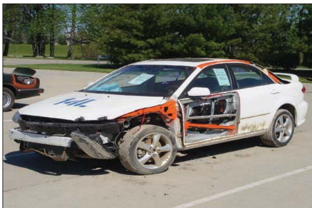
Fig. 34–6. Notice the reinforcements revealed in the cutouts on a Mazda 6.
