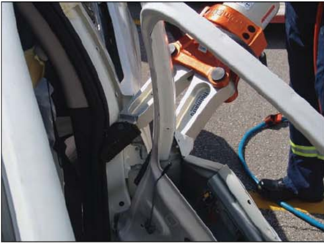
Fig. 34–8. Removing the door by tearing the door from the latch
