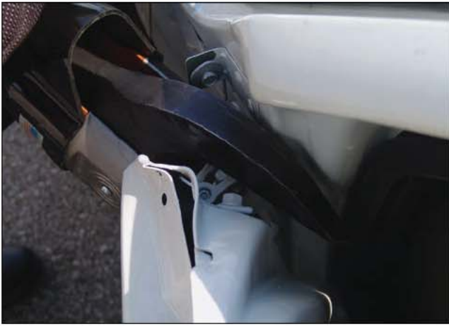
Fig. 34–59. Cutting the door hinge—close-up
