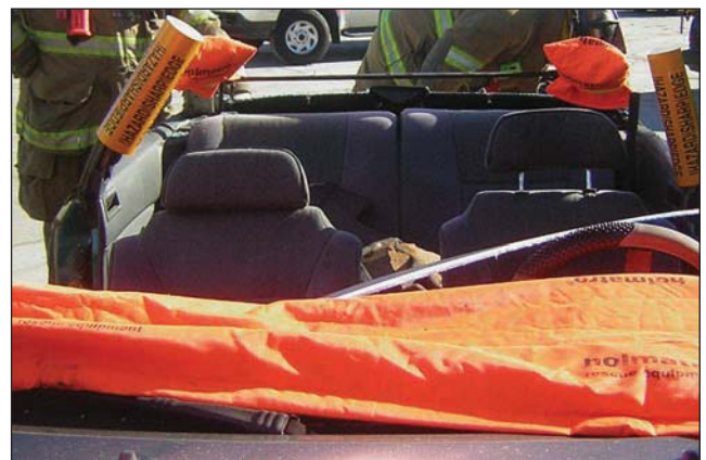
Fig. 34–37. It is very important to cover all sharp edges with some sharps covers.
