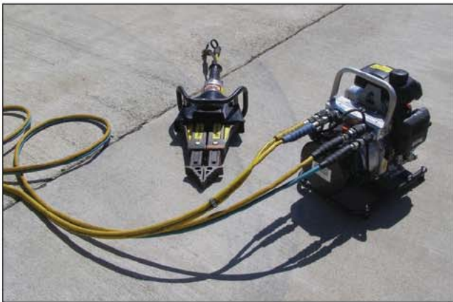
Fig. 34–23. The photo displays a spreading tool and power unit.
