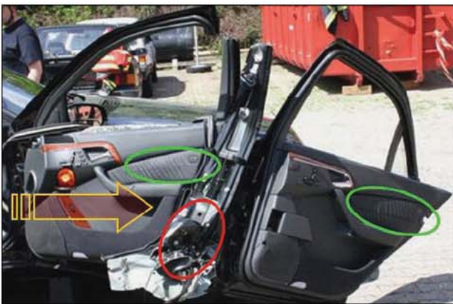
Fig. 34–60. Debris with live SRS
