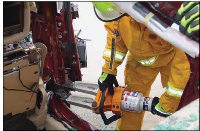
Fig. 34–62. With the purchase point made, use the spreaders to tear the B-post off.
