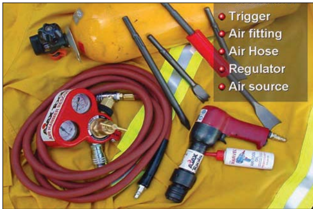
Fig. 34–26. The air tool displayed is an Ajax tool.
