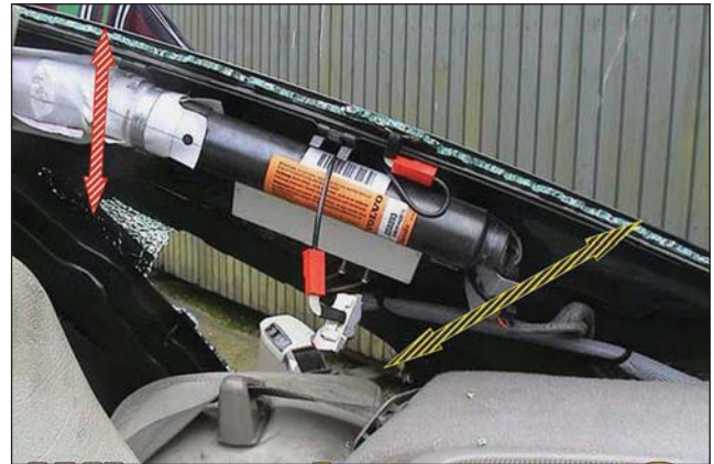
Fig. 34-17. Once the trim is stripped back, locate and cut around side curtain cylinder.
