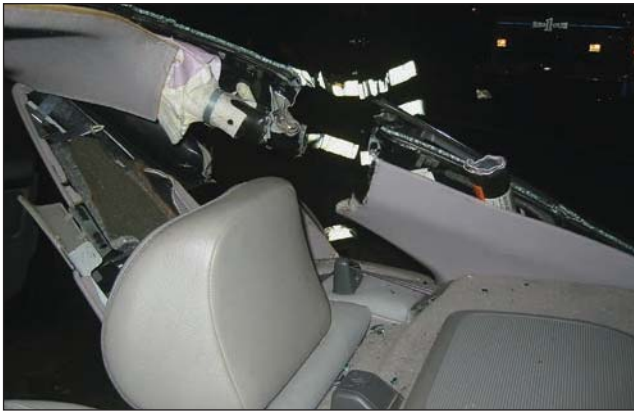
Fig. 34-15. An accidental cut of live side curtain cylinder could be extremely dangerous for both the rescuer(s) and the patient(s).
