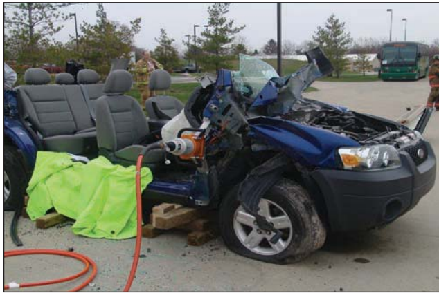
Fig. 34–5. Notice relief cut behind the fender on this 2007 Escape Hybrid.
