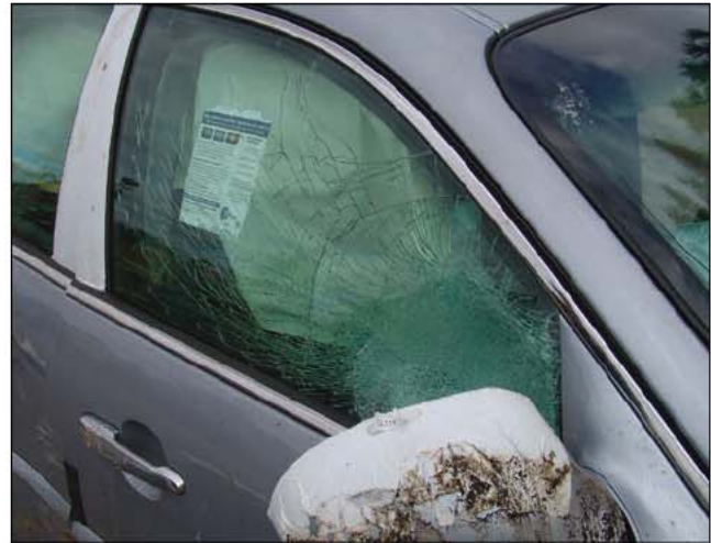
Fig. 34–9. Notice how the laminated side glass (EPG) in this photo is shattered worse at the point of impact.
