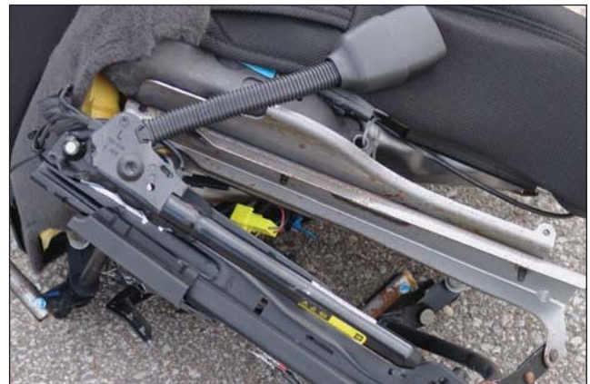
Fig. 34-18. The buckle side seat belt pretensioner is shown here.
