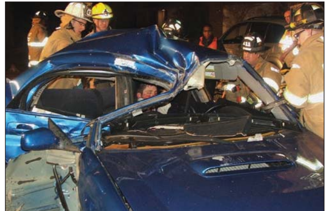
Fig 34–39. After securing the scene and hazards are mitigated, the victim is secured and a pathway is created to extricate the patient.
