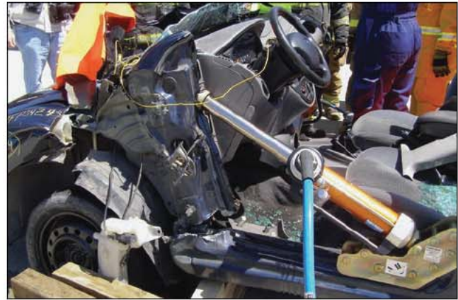
Fig. 34–69. A ram in place to perform a dash roll
