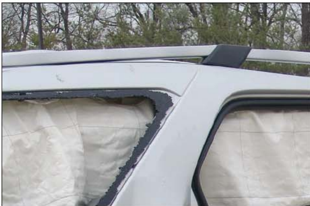
Fig. 34–13. Notice how both the Taurus side curtain and side impact bag were deployed.
