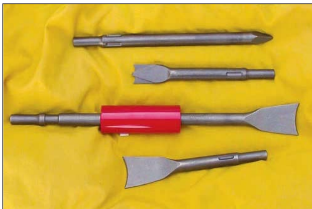
Fig. 34–27. A variety of Air chisel bits are good to have on hand to be used in many instances.
