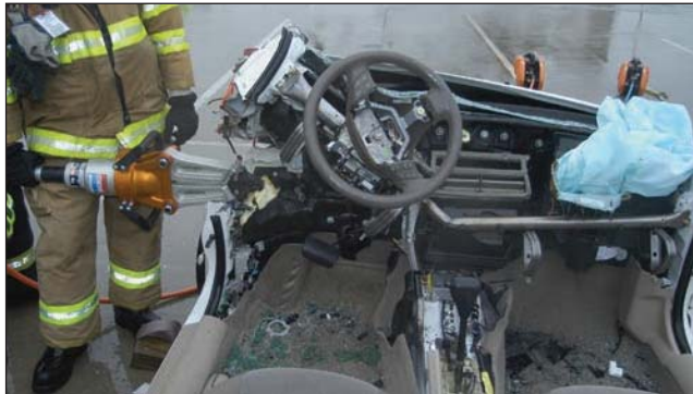
Fig. 34-63. After a relief cut is made, begin using a spreader to begin the end dash lift.
