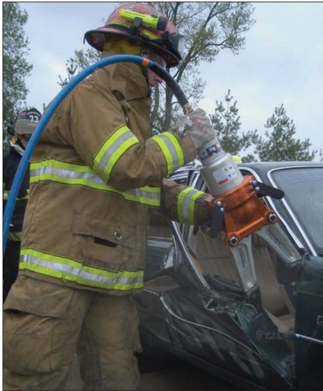
Fig. 34–55. Spreading the front of a door to remove the door by pulling the hinges off.
