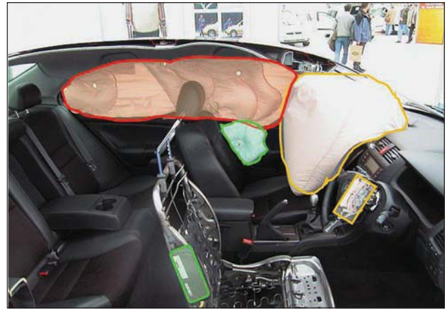
Fig. 34–48. This photo shows typical SRS locations deployed and undeployed.
