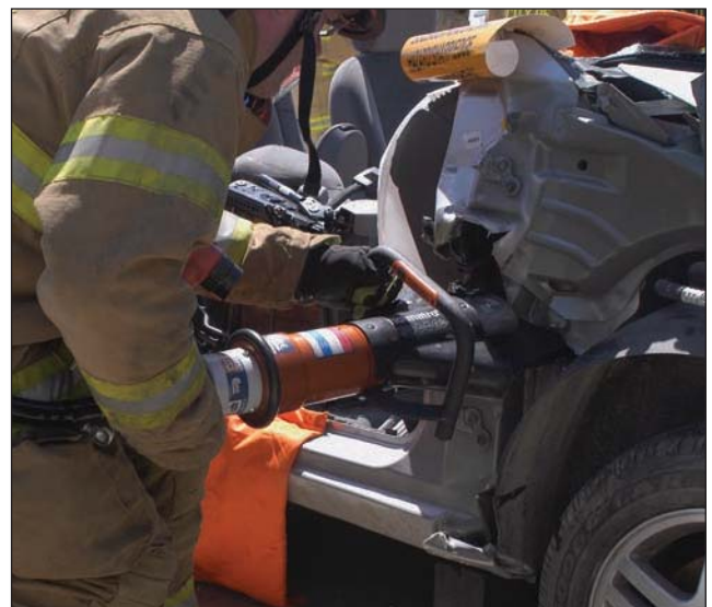
Fig. 34-66. Making a dash relief cut
