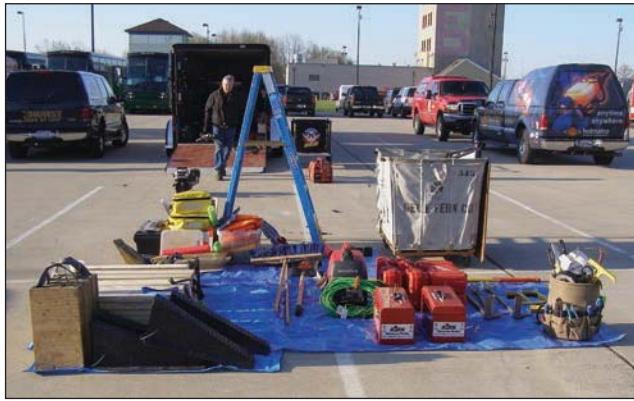
Fig. 34–21. Pictured above is a typical tool staging as used on a MVC. This allows tools to be quickly and easily identified and retrieved when needed.
