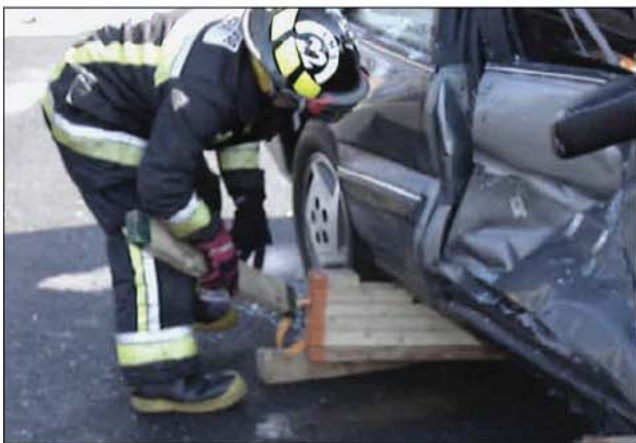
Fig. 34–44. It is critical to stabilize any vehicle in which extrication is involved.
