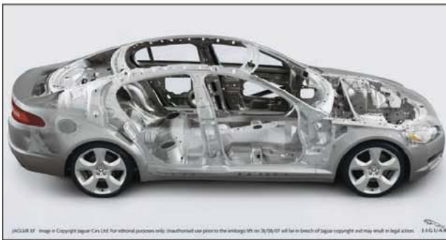
Fig. 34-3. This photo reveals the space-frame construction in a new vehicle.
