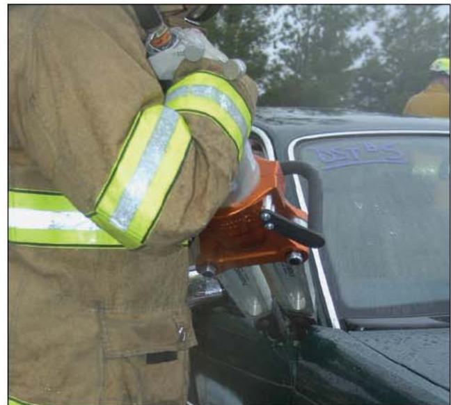
Fig. 34–54. Making a purchase point to remove the door at the hinge location
