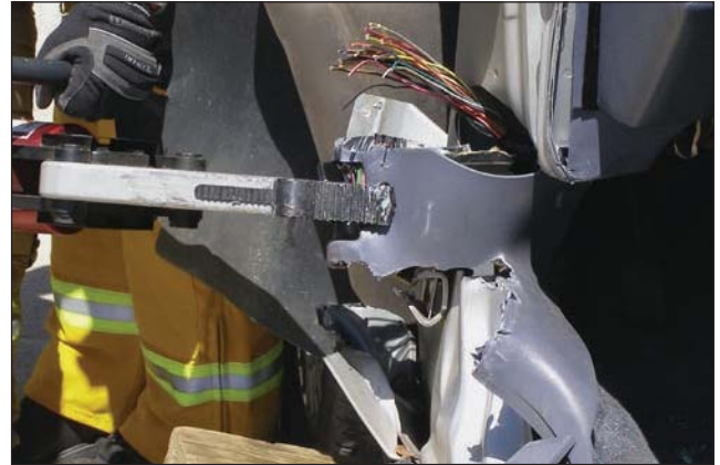
Fig. 34-65. As relief cuts are made, pull the tab back.
