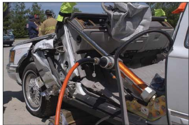
Fig. 34–70. Notice how the dash rolls upward and forward.
