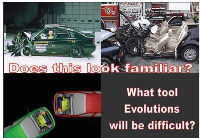
Fig. 34–49. The vehicle crumple zones are similar in most high-energy crashes.
