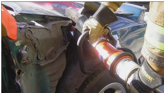
Fig. 34-64. Use the crumple zone cut to isolate the dash from the rest of the vehicle.
