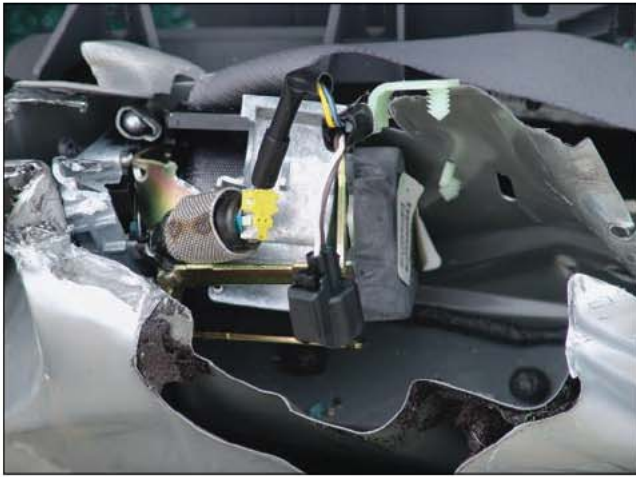
Fig. 34–19. The spool side seat belt pretensioner is shown in this photo.
