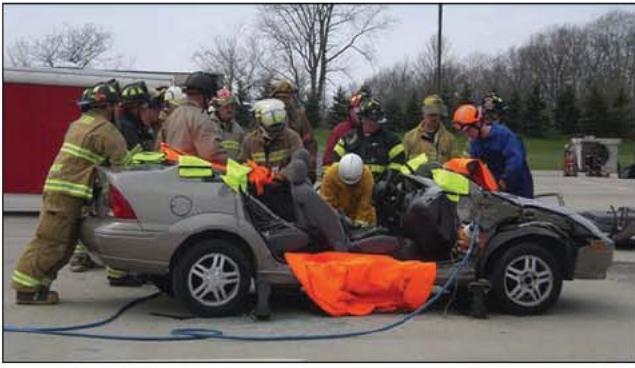
Fig. 34–38. There are many ways to cover sharps from old hose sections to manufactured sharps covers.
