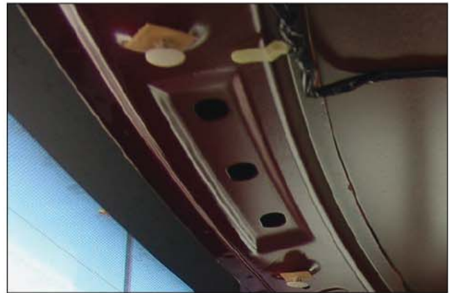
Fig. 34–14. With the trim of the 2007 Fusion removed, the undeployed side curtain is revealed.
