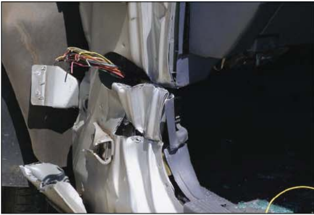
Fig. 34–67. This photo displays dash lift relief cuts.
