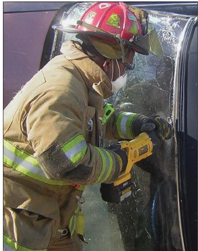
Fig. 34–10. Many departments now use reciprocating saws in their glass management.
