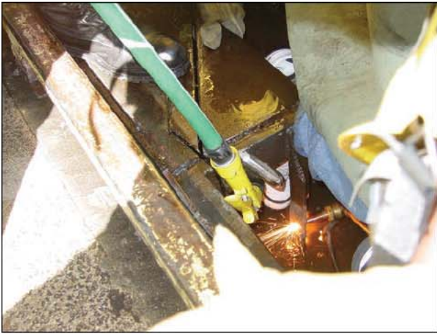
Fig. 35–78. A cutting torch can prove to be an effective way to extricate a victim trapped in heavy machinery.
