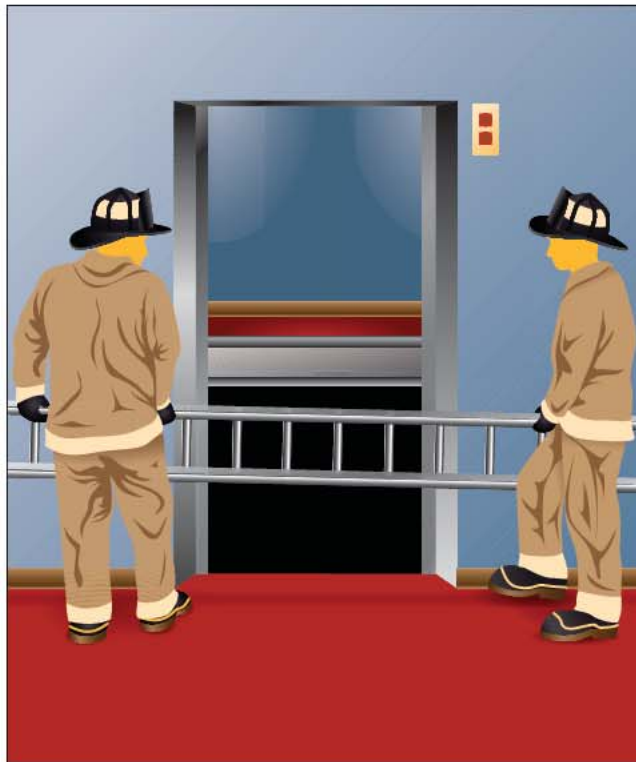
Fig. 35–86. A roof or attic ladder is held across the opening to prevent people from falling down the shaft as they are removed from the elevator car.
