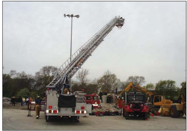
Fig. 35–20. Aerial ladders can be used at technical rescue incidents as observation towers.
