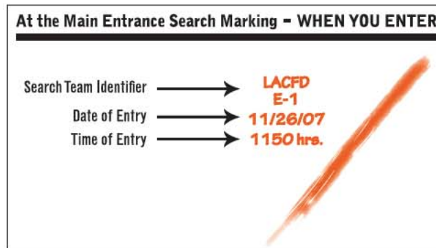
Fig. 35–30. Place these search markings at the main entrance when you enter.
