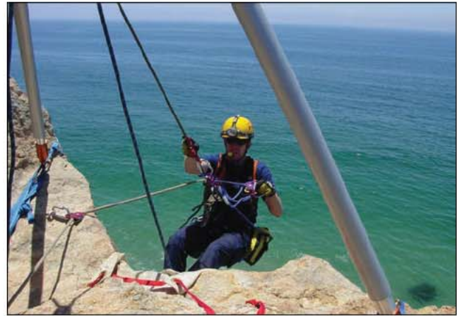
Fig. 35–44. For safety purposes, two ropes should be used when possible, especially when raising victims and/or rescuers.
