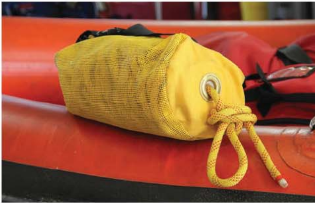
Fig. 35–11. Throw bags for water rescue include a foam flotation ring at the bottom of the bag (shown inside the metal grommet).
