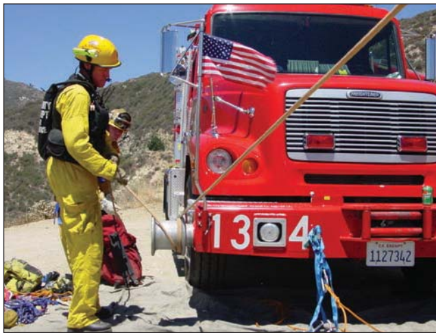
Fig. 35–46. Capstans are used in combination with winch systems and offer additional rescue options.
