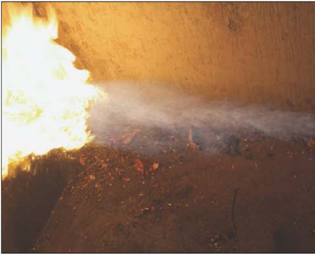
Fig. 5–5. When an ignitable liquid is atomized it becomes easier to vaporize and ignite.
