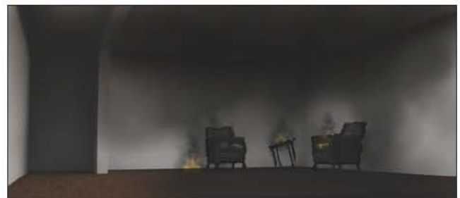
Fig. 5–10. The four stages of fire development: ignition, growth (pre-flashover), fully developed (flashover), and decay (post-flashover)
