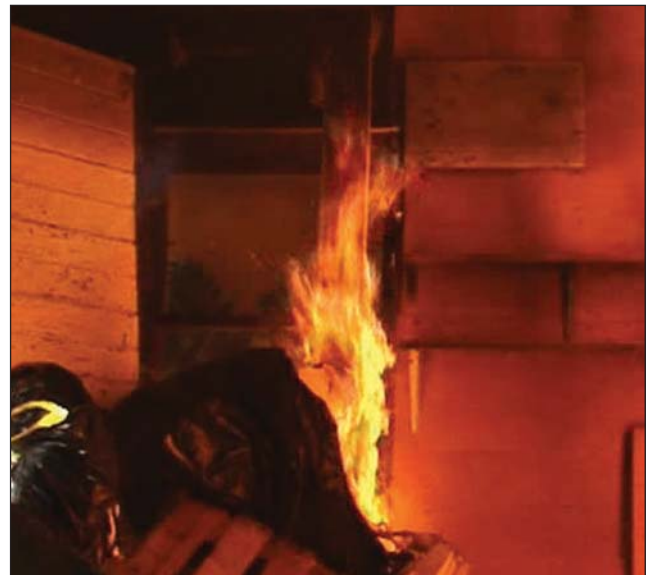
Fig. 5-8. As flame passes over the surface of a material, it can ignite the material.
