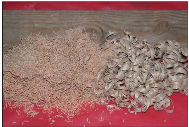
Fig. 5-4. Each of these items is wood: the block, the shavings, and the sawdust. But they each have a different physical configuration and a different surface-area-to-mass ratio that will make ignition easier or more difficult.
