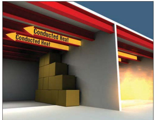
Fig. 5-7. A steel beam exposed to fire in one room can ignite materials in an adjacent room.
