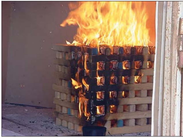
Fig. 6–10. Establishing the rating of an extinguisher often involves the use of wood crib test fires. (Courtesy of Tom Jenkins)
