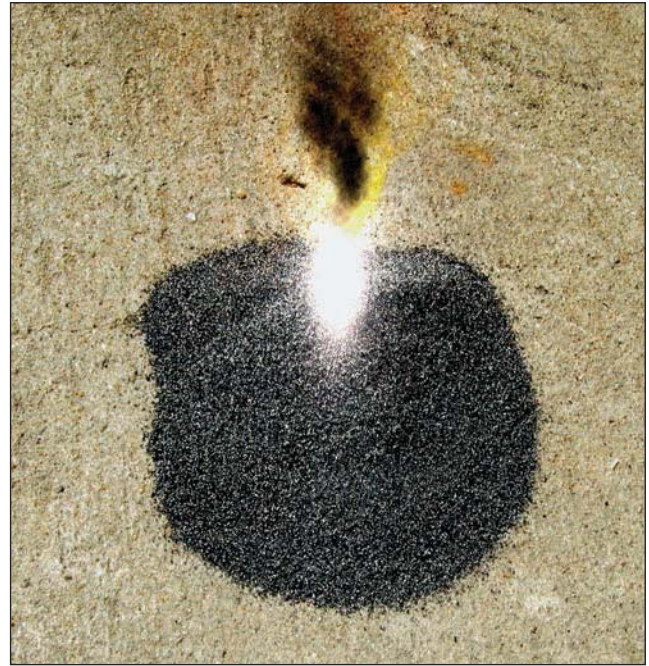
Fig. 6–12. Applying dry powder to a Class D fire is risky and requires the fire extinguisher operator to monitor the situation for “hot spots” that might flare up.
