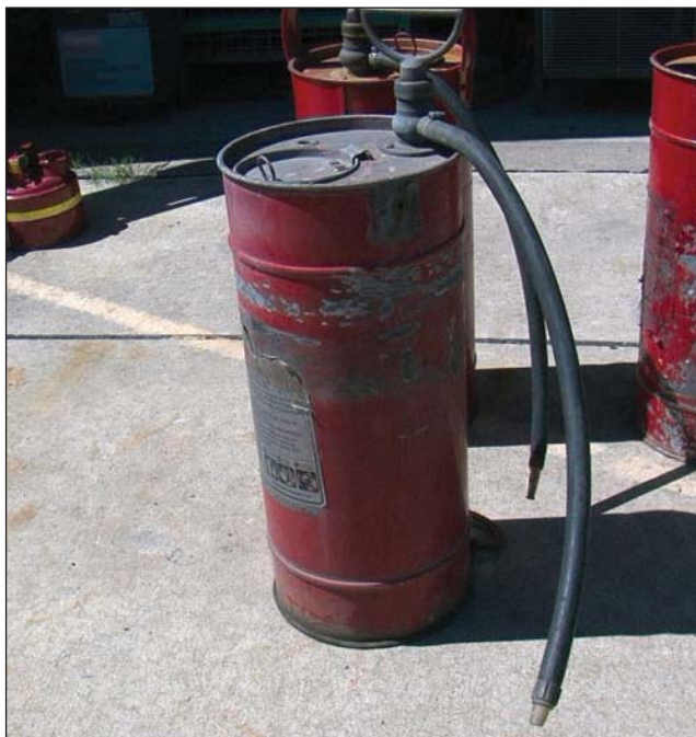
Fig. 6–7. Pressure can be generated for fire extinguishers through storing the pressure in the main cylinder, having an outside cartridge, or through a manual pump.
