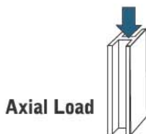
Fig. 7-6. An axial load is imposed on the column as the load passes through the center of the column.
