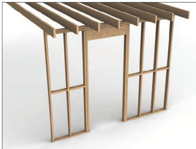
Fig. 7-2. The studs supporting the floor joists in this wood-frame wall are in compression.
