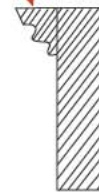
Fig. 7-7. The parapet wall is eccentrically loaded with a cornice (a decorative wall projection attached to the top of many apartment buildings.) This load does not pass through the center of the wall.
