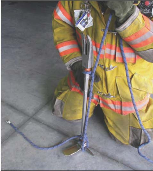
Fig. 8–20. Using a clove hitch and a half hitch, along with a tag line, you can successfully raise a Halligan tool to an upper floor.
