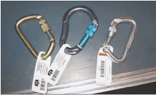
Fig. 8–34. A carabiner is the most common rope tool used in the fire service. When used in conjunction with a length of rope or webbing, it can create an emergency firefighter escape system.
