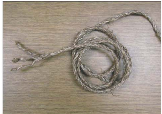
Fig. 8–3. Laid or twisted rope construction involves the twisting of three strands of natural or synthetic rope.
