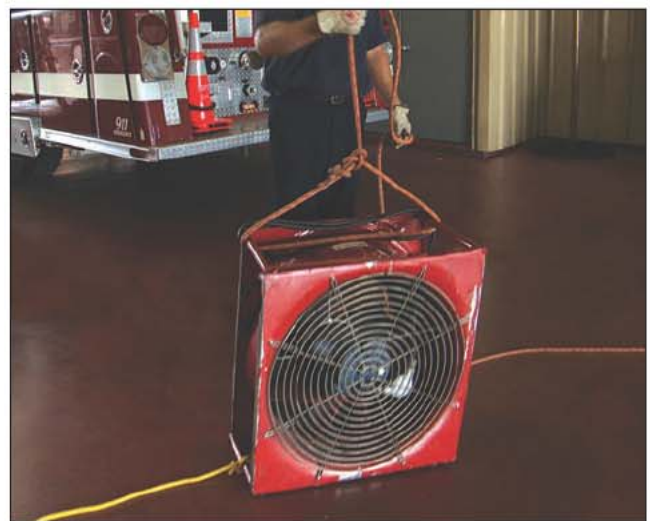
Fig. 8–22. A bowline tied around the top of an exhaust fan, along with a clove hitch for a tag line, can allow the fan to be hoisted to an upper floor.
