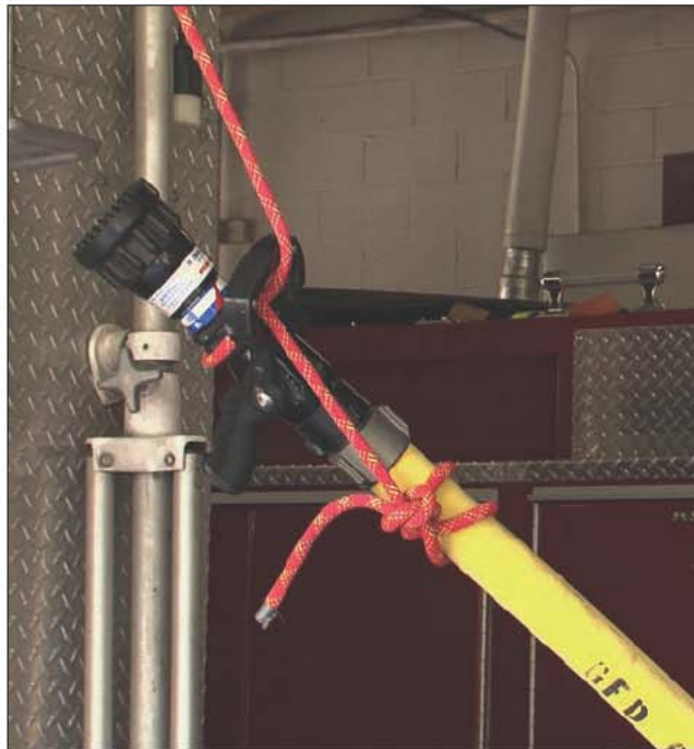
Fig. 8–23. A hose line can be hoisted by tying a clove hitch below the first coupling.
