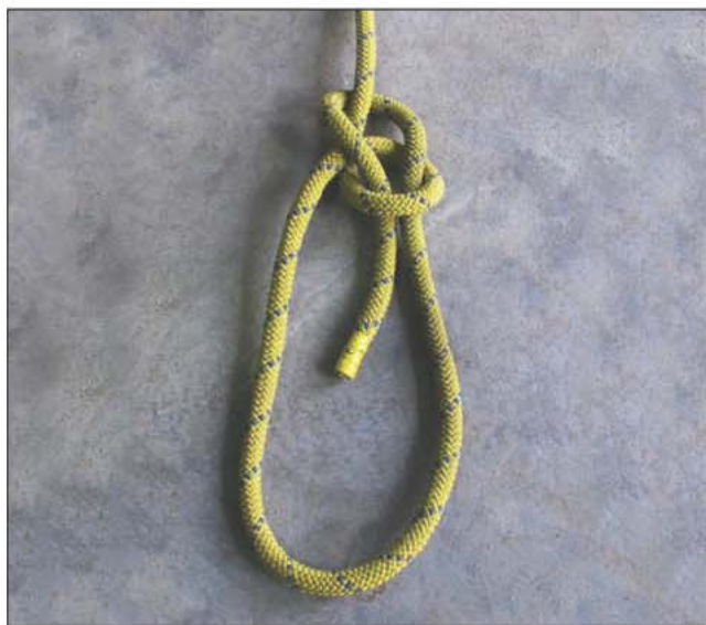
Fig. 8–13. A bowline forms a secure knot when tension is applied to the rope.
