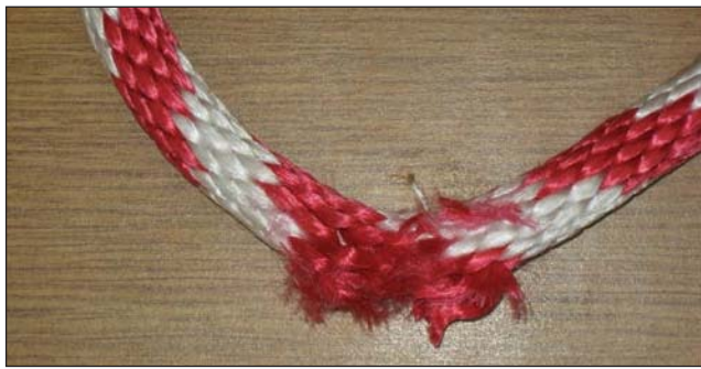
Fig. 8-4. Braided rope is commonly found in synthetic rope used by the fire service. A drawback of this type of rope is that all strands are exposed to damage from abrasion.
