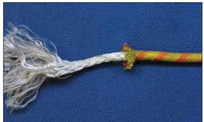
Fig. 8-6. Kernmantle rope is the most common fire service rope since it is designed for life safety operations.
