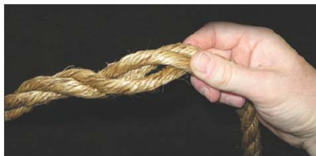
Fig. 8–29. Untwist the strands of twisted or laid rope to inspect.
