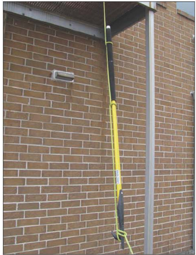
Fig. 8–21. Usually one half hitch and a clove hitch can secure a pike pole to be hoisted.
