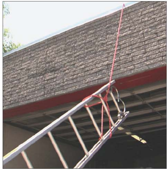
Fig. 8–24. Firefighters using a bowline and a clove hitch to hoist a ladder.
