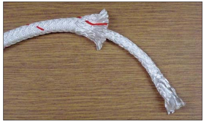
Fig. 8-5. Braid-on-braid rope has many of the same drawbacks as simple braided rope, except that the outer core creates a protective "jacket" for the rope.
