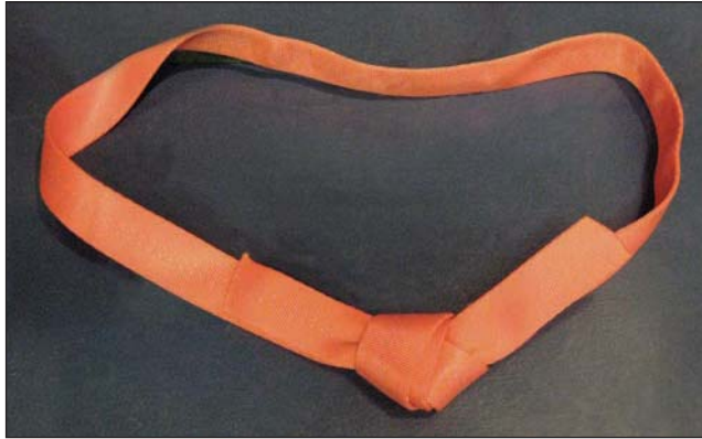
Fig. 8–17. A water knot is typically used to tie ends of webbing together.
