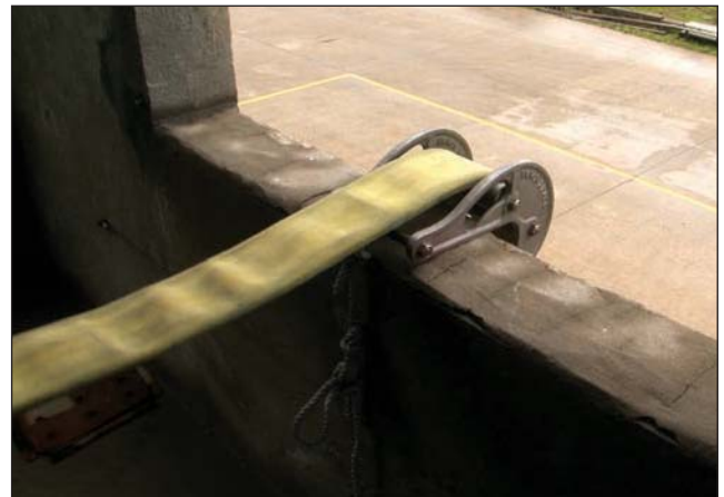
Fig. 8–19. Hose rollers can be used to protect hose and rope when drawn over sharp edges.
