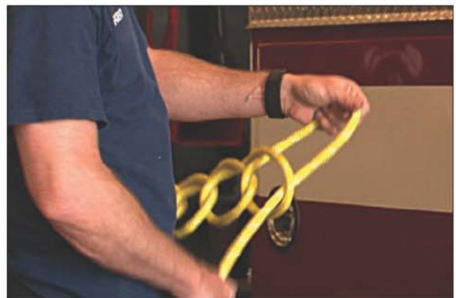
Fig. 8–31. If you don't have a mesh bag, tie the rope in a daisy chain before placing it into a washing machine. See your Skill Drill book for steps to create a daisy chain.
