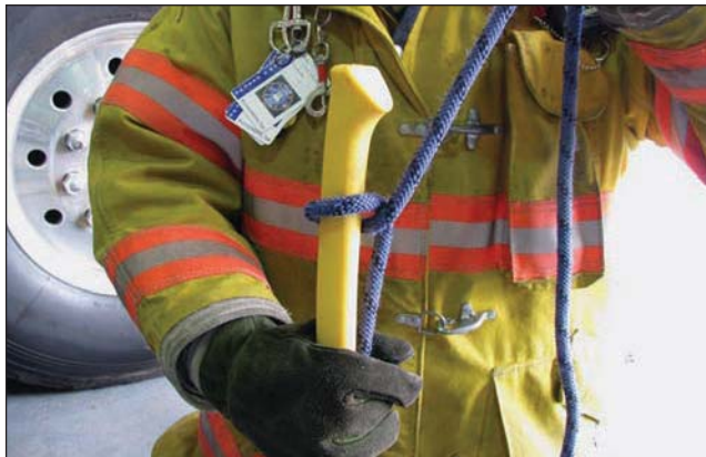
Fig. 8-10. A half hitch being used to hoist an axe
