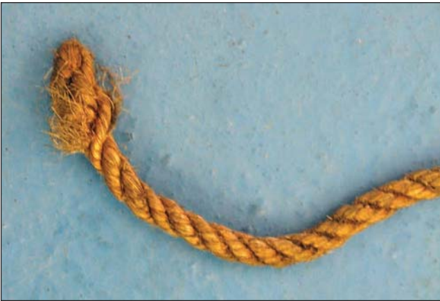
Fig. 8–1. Natural fiber rope is made from organic materials and isn't generally used for fire or rescue purposes.
