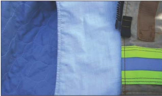
Fig. 9-11. The three layers of structural PPE—Thermal liner with the moisture barrier and outer shell of a structural coat
