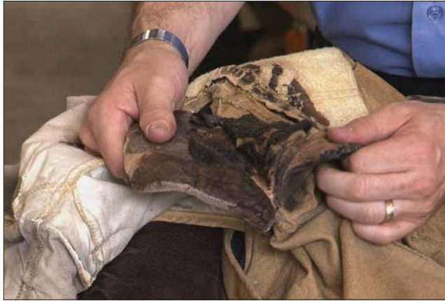
Fig. 9–24. Damaged gear being inspected
