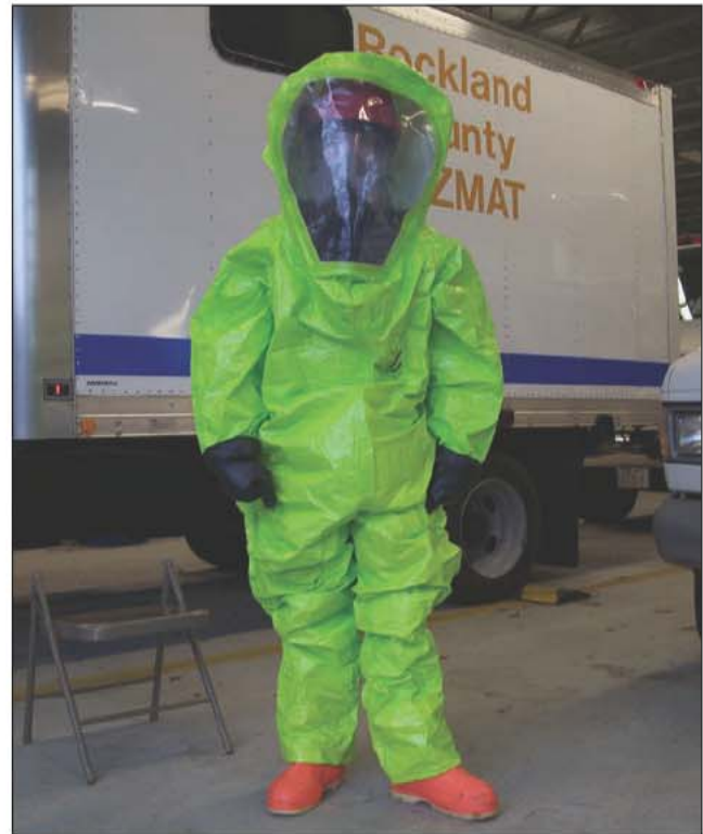
Fig. 9-6a. Level A hazardous material PPE—This is the highest level of protection, with integrated gloves and boots. They come in different materials for protection against different chemicals. SCBA is donned under the suit for respiratory protection. (Courtesy of Jerry J. Knapp)
