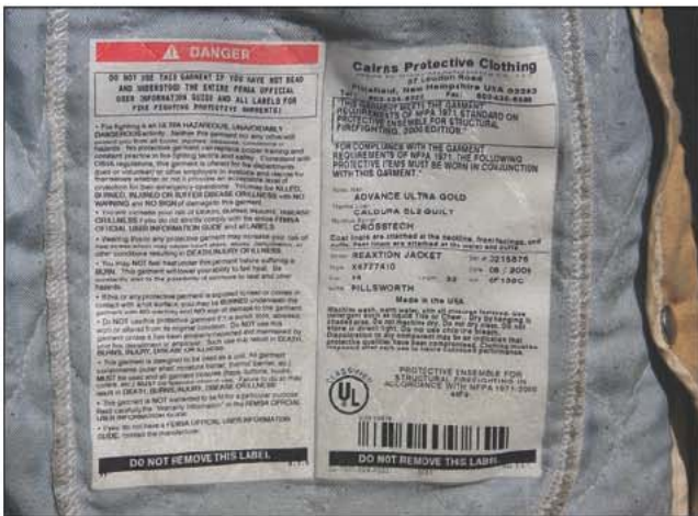
Fig. 9-12. The required NFPA label with the garment's information
