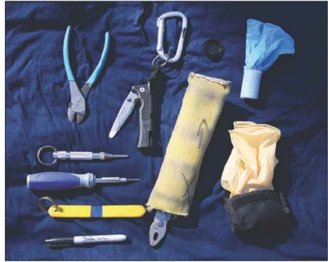
Fig. 9–23. Personal tools—your personal tools should include some combination of extra medical gloves (in a holder or even a 35 mm film case), wire cutters, screwdriver, pliers, center punch, and a knife. They can be used while performing your duties, or even to rescue yourself in an emergency.
