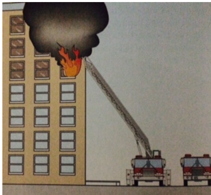
Figure 9 - Aerial apparatus positioned inside the pumper.
