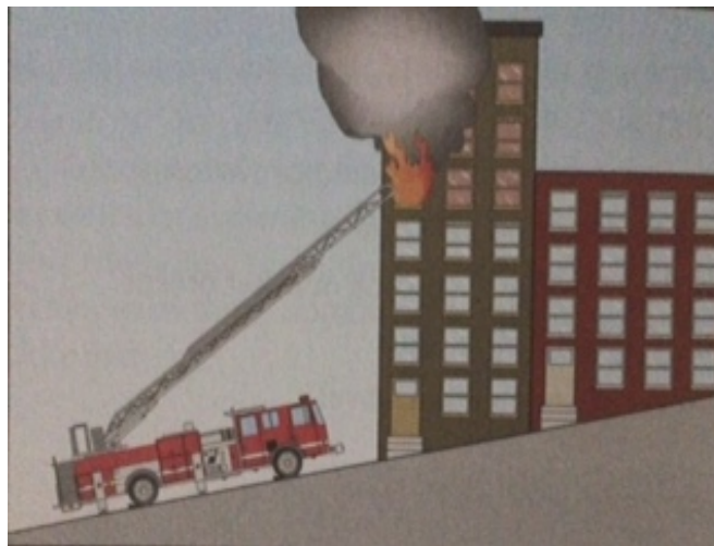
Figure 10 - Aerial device positioning when approaching from the downhill side.
