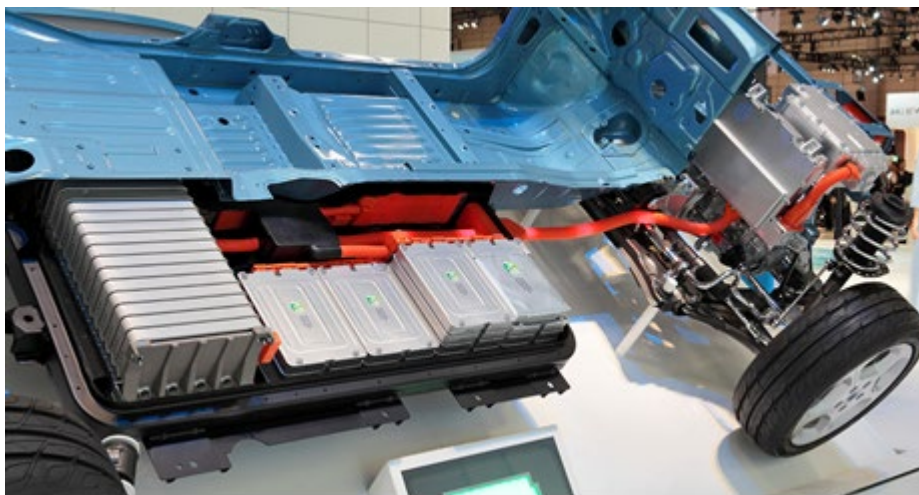
Figure 11. Battery Banks for Electrical Vehicles
