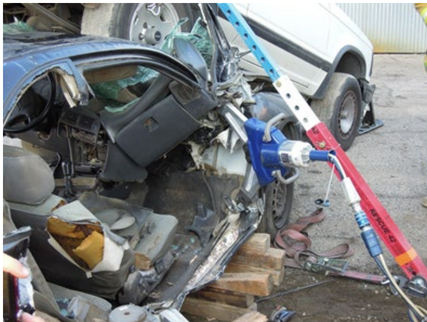
Figure 7. Dash displacement with stabilization of vehicle on top
