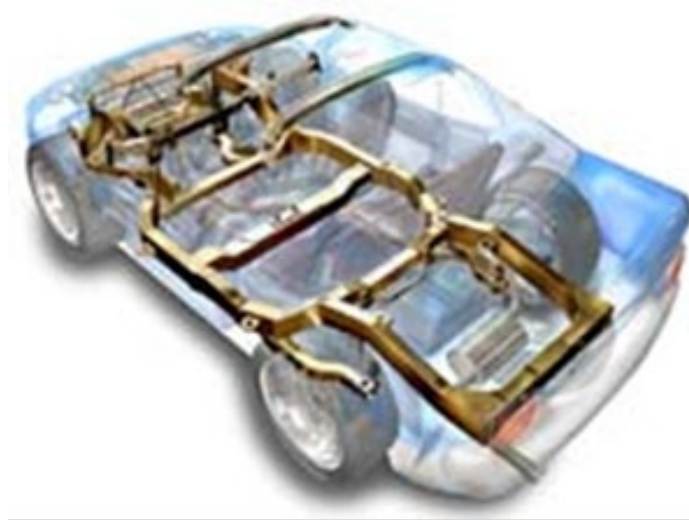
Figure 2. Full Frame Construction
