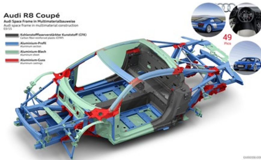
Figure 4. Space Frame Construction
