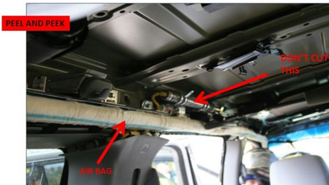
Figure 8. Peel and peek for hidden hazards
