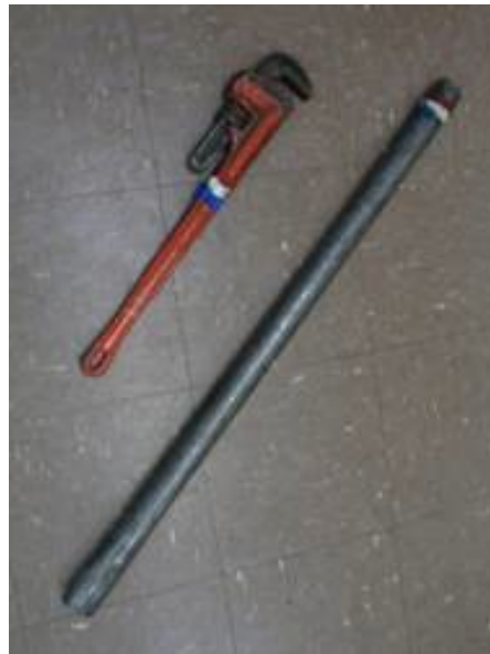
Figure 18 - Pipe wrench used like vice grips to twist off lock face and expose internal locking mechanism
