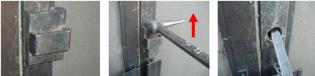
Figure 144 - Insert K tool, pry up on lock cylinder, slide key tool in and unlock
