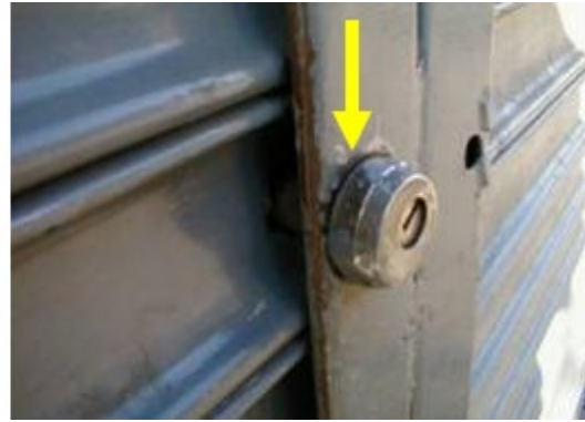
Figure 187 - Downward pressure to snap the brass pin
