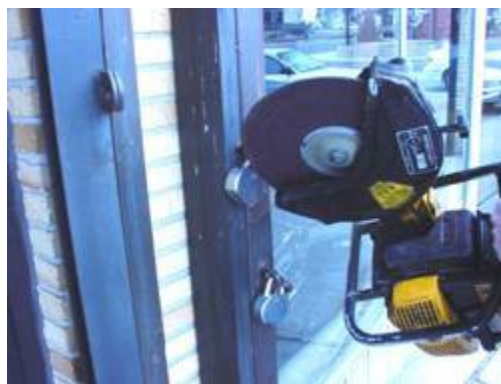
Figure 164 - Cut shackle with Rotary saw
