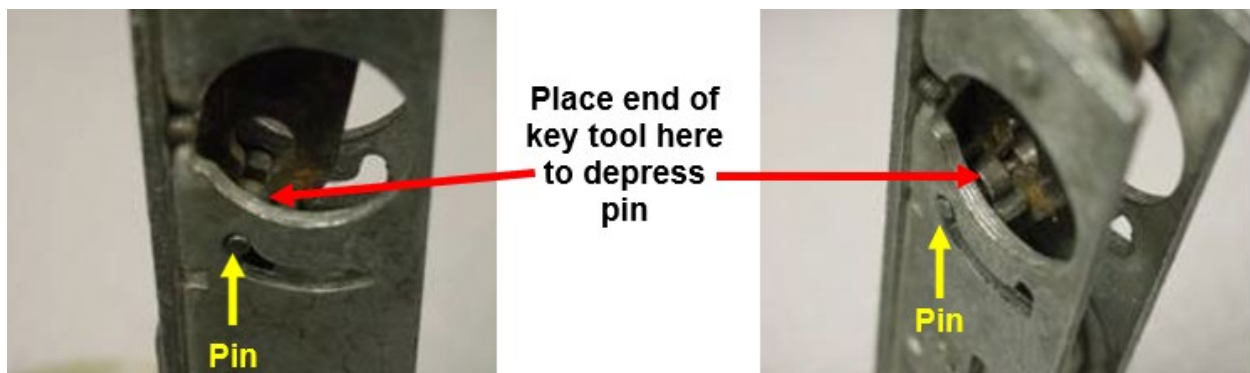
Figure 145 - Place end of key tool in to depress the pin
