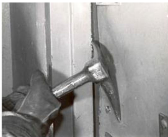
Figure 63 - Gapping the door with the ADZ
