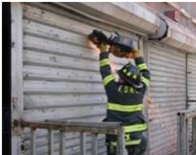
Figure 193 - Do not cross cuts until second cut is complete
