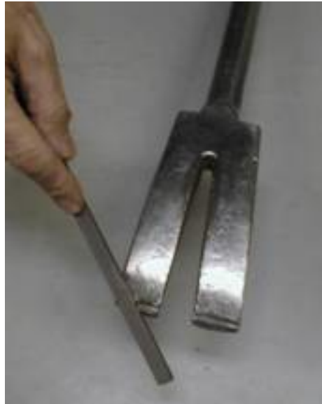
Figure 8 - Sharpen the bevel of the forks
