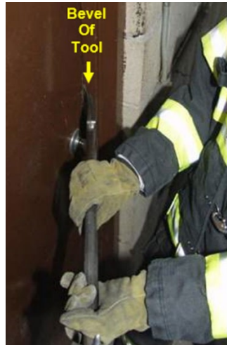
Figure 64 - Bevel to the frame
