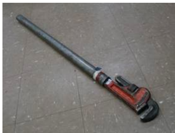
Figure 19 - Pipe can be slid onto the pipe wrench and used as a cheater bar to gain leverage on sticky locks
