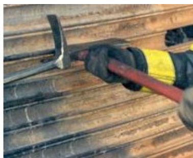
Figure 197 - Drive the Pike end of the Halligan into a slat to remove. If slats are tight, drive the Halligan with an axe.
