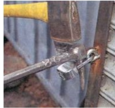
Figure 169 - When striking either tool with the axe, the eight-pound axe is preferred.
