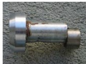
Figure 158 - Bolt lock front and side views
