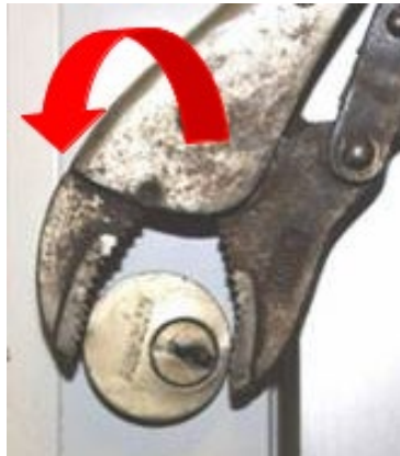
Figure 147 - Unscrew cylinder to expose locking pin
