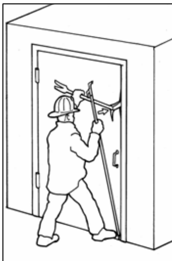
Figure 220 - Utilize the hook as a force and hit the halligan
