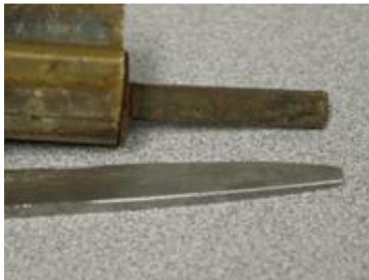
Figure 134 - Proper end of key tool
