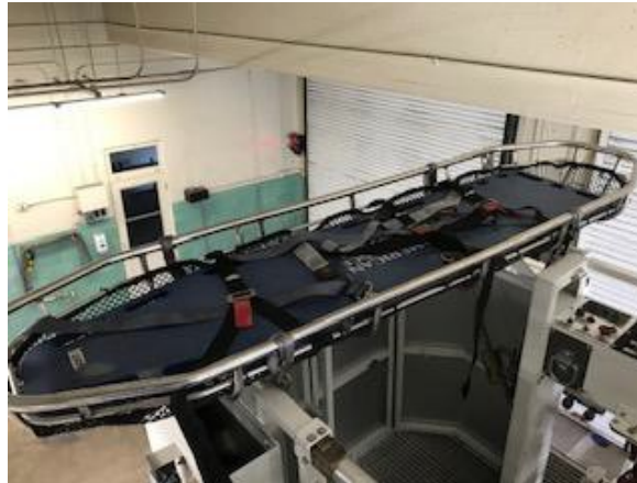
Figure 14 - Stokes litter attached to the aerial tower
