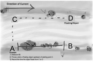
Current = Distance AB (Meters)/Time CD (Seconds) 1 foot per second equals .59 knots 1.69 feet per second equals 1 knot
